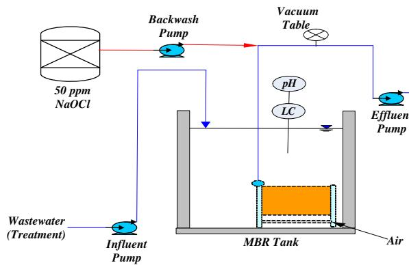
Fig. 1. Schematic diagram of the MBR pilot reactor.
