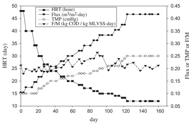
Fig. 4. Variation of operation parameters in the MBR system.
