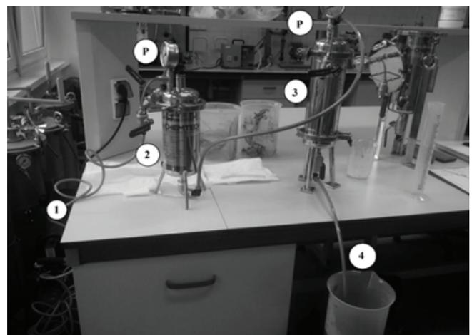
Fig. 2. Research station for overpressure filtration (1, air compressor; 2, displacement tank; 3, tank containing filter; 4, filtrate tank; and P, pressure gauge).
