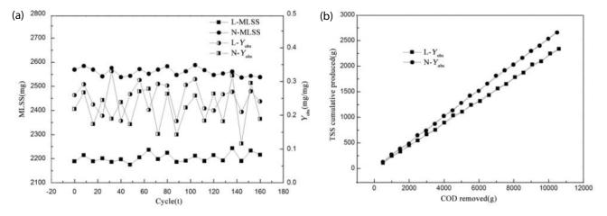
Fig. 2. Sludge observed yield  $(Y_{obs})$  in both the reactors. (a) Daily sludge concentration and sludge observed yield  $(Y_{obs})$  and (b) cumulative sludge observed yield  $(Y_{obs})$ .
