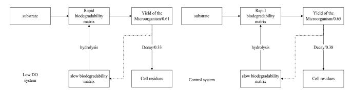
Fig. 7. Analysis of the biomass balance under different DO.
