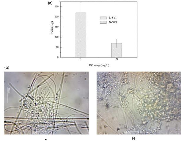
Fig. 3. (a) SVI of the sludge under different DO and (b) optical micrographs of the sludge under different DO. Samples L denotes sludge samples from the low-DO system and N denotes sludge samples from the control system.
