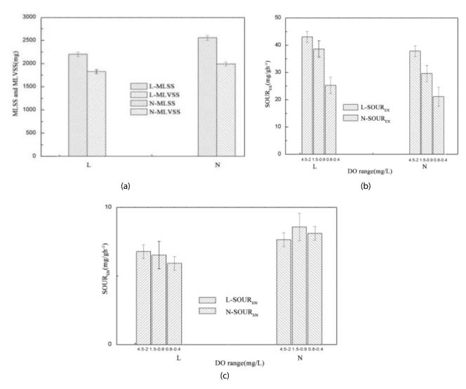
Fig. 4. (a) SS/VSS of the sludge under different DO, (b) SOUR<sub>EN</sub> of the sludge under different DO, and (c) SOUR<sub>EN</sub> of the sludge under different DO. Samples L denotes sludge samples from the low-DO system and N denotes sludge samples from the control system.
