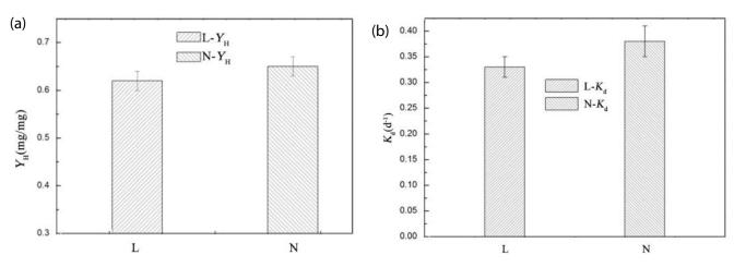
Fig. 5.  $Y_{\mu}$  of the sludge under different DO and (b)  $K_{d}$  of the sludge under different DO.
