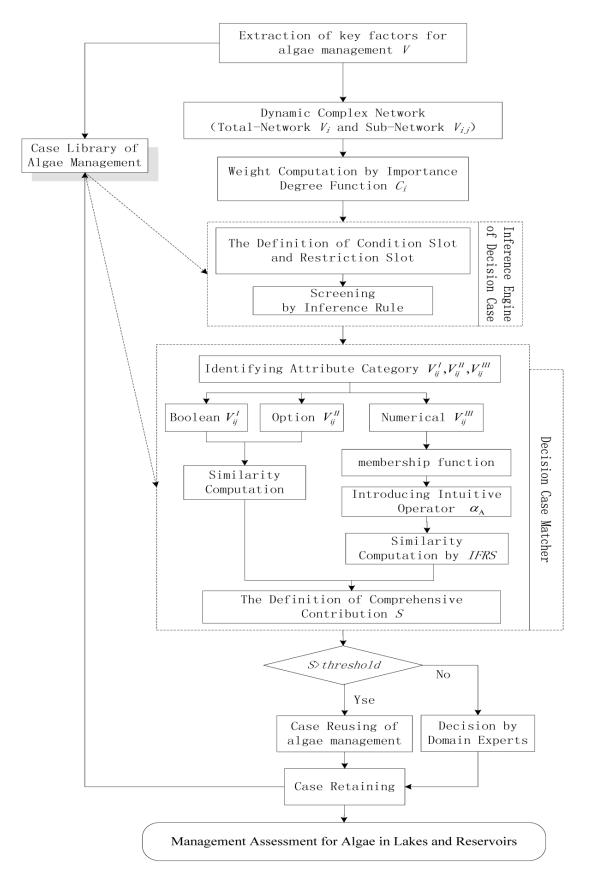
Fig. 2. Working flow of CBR-OSS model.
