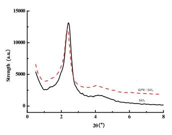
Fig. 3. XRD spectrum of mesoporous SiO<sub>2</sub>, KPW/SiO<sub>2</sub>.
