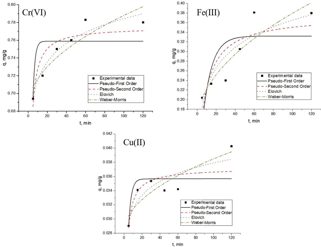
Fig. 12. Kinetics of the metal adsorption using *Saccharomyces cerevisiae* in Cr(VI)-Fe(III)-Ni(II)-Zn(II)-Cu(II) system.
