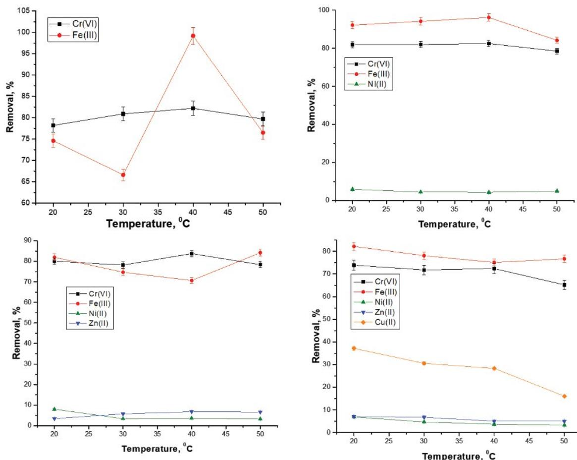
Fig. 6. Effect of temperature on the sorption of metal ions by *Saccharomyces cerevisiae* biomass (at  $T$ : 20°C; sorbent dosage: 0.5 g L<sup>-1</sup>; and adsorption time: 1 h).
