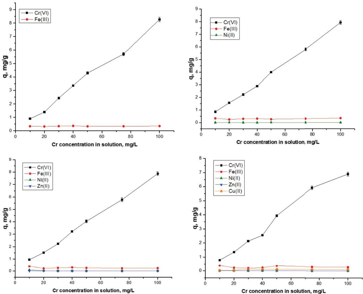
Fig. 13. Removal of metal ions at different chromium concentration in solution (at  $T$ : 20°C; sorbent dosage: 0.5 g L<sup>-1</sup>; and adsorption time: 1 h).
