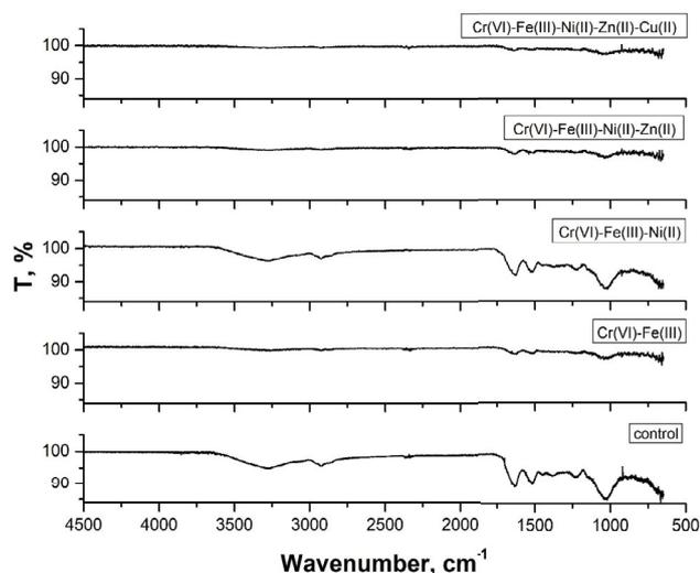
Fig. 2. FTIR spectrum of *Saccharomyces cerevisiae* biomass before and after metal biosorption.
