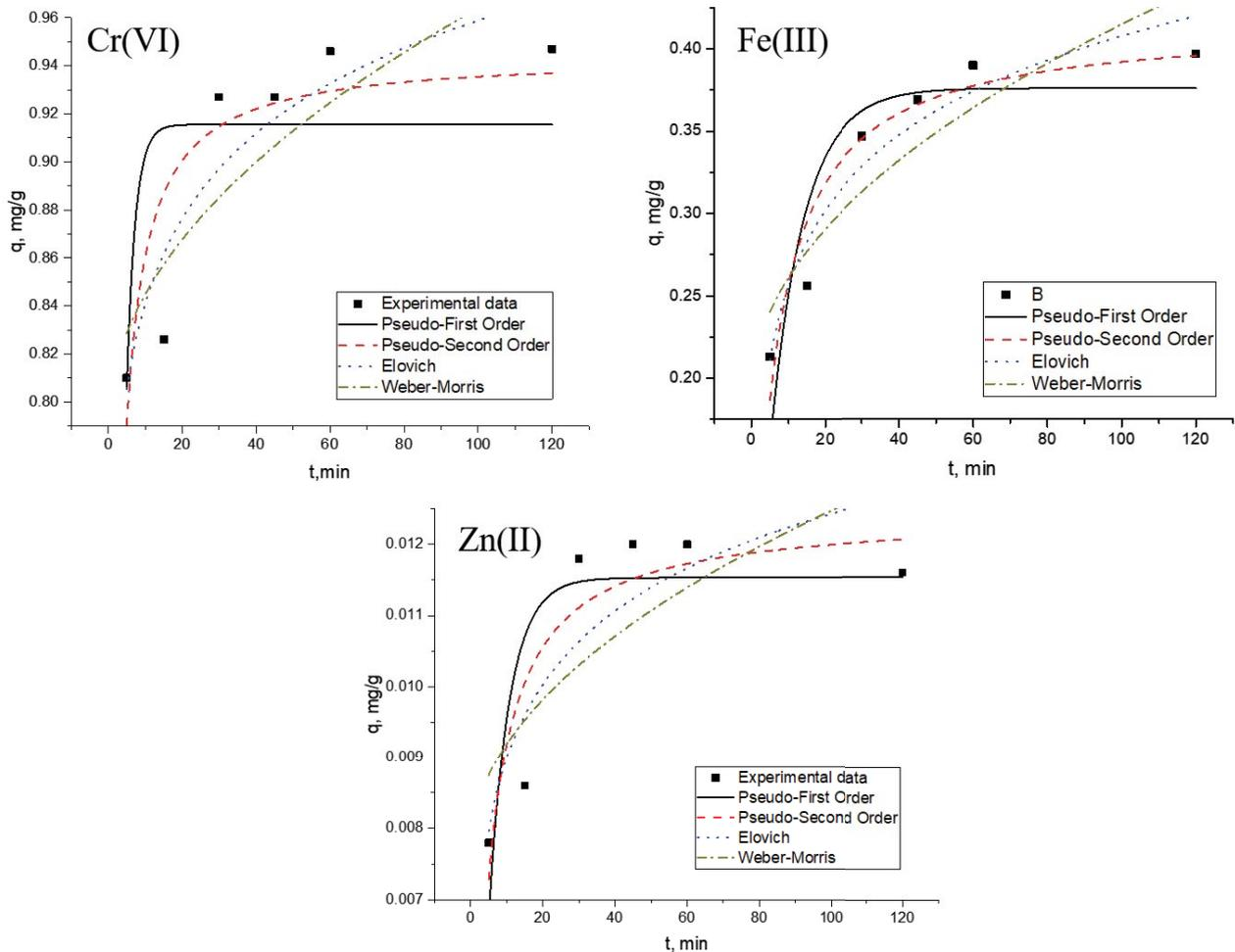
Fig. 11. Kinetics of the metal adsorption using *Saccharomyces cerevisiae* in Cr(VI)-Fe(III)-Ni(II)-Zn(II) system.
