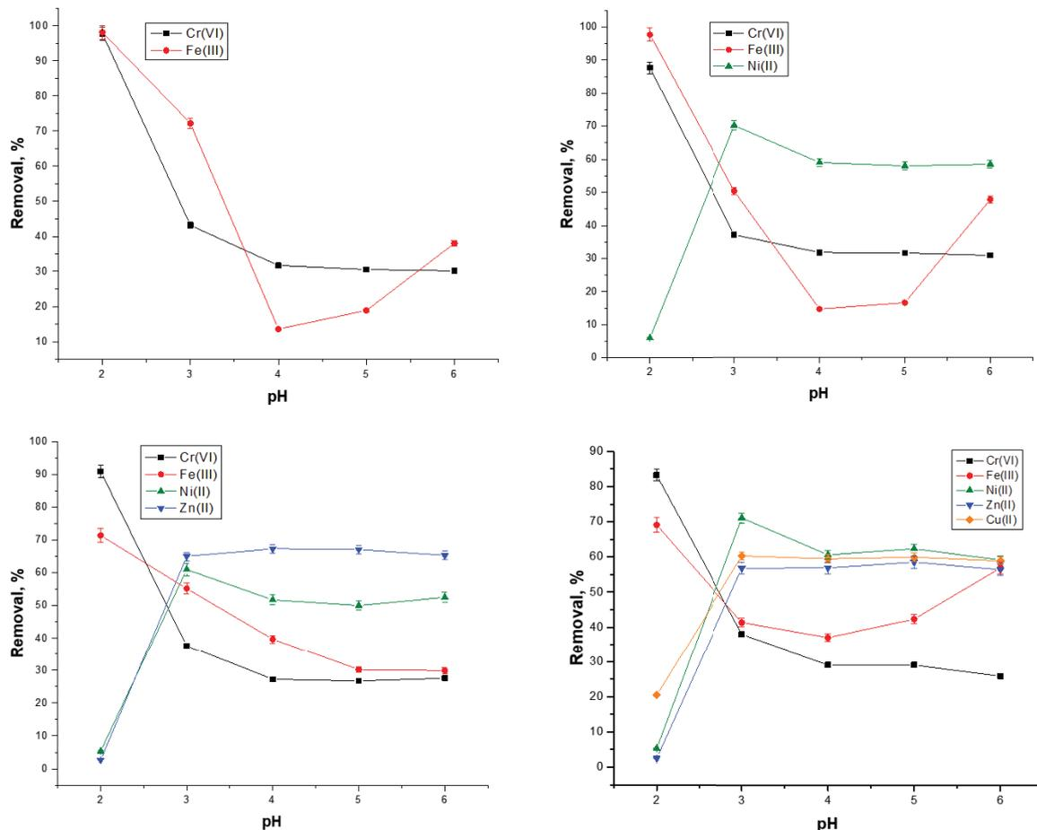
Fig. 5. Removal of metal ions at different initial pH (at  $T$ : 20°C; sorbent dosage: 0.5 g L<sup>-1</sup>; and adsorption time: 1 h).
