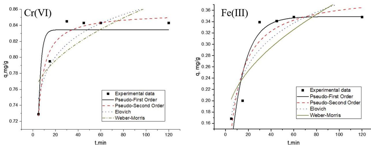
Fig. 10. Kinetics of the metal adsorption using *Saccharomyces cerevisiae* in Cr(VI)-Fe(III)-Ni(II) system.
