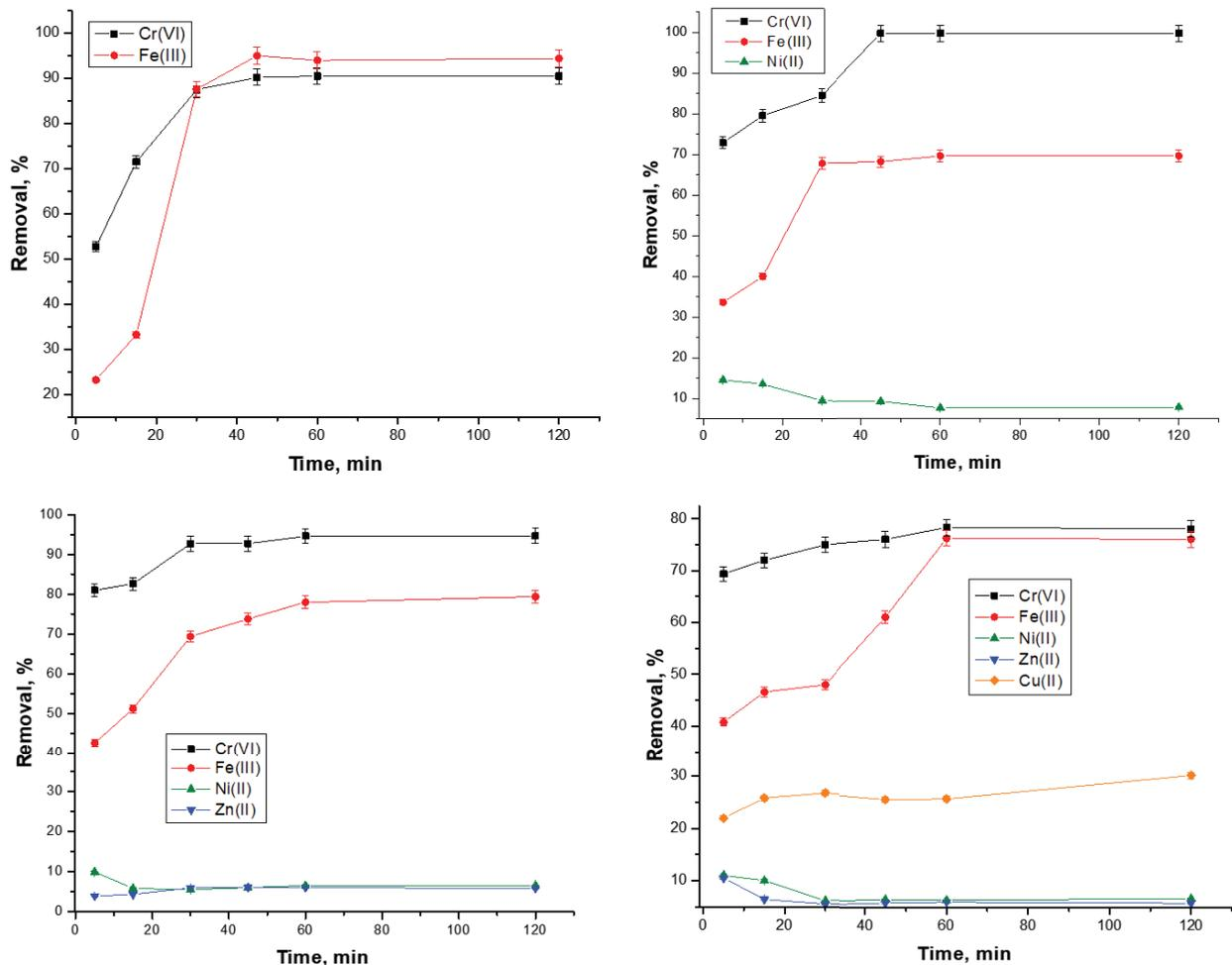
Fig. 8. Adsorption of metal ions on *Saccharomyces cerevisiae* as the function of time (at  $T$ : 20°C and sorbent dosage: 0.5 g L<sup>-1</sup>).
