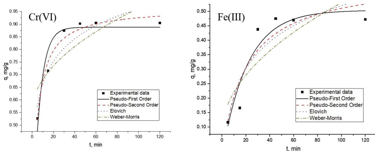
Fig. 9. Kinetics of the metal adsorption using *Saccharomyces cerevisiae* in Cr(VI)-Fe(III) system.
