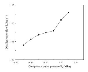
Fig. 8. Distillate flow rate as a function of discharge pressure.
