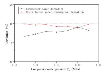
Fig. 10. Variation of experimental deviation with changes in discharge pressure.
