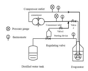
Fig. 3. Experimental system diagram.
