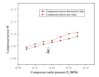
Fig. 7. Compressor power as a function of discharge pressure.
