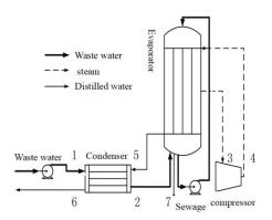
Fig. 1. MVR method to treat the water co-produced with oil design model.
