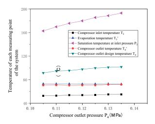
Fig. 6. Effect of discharge pressure on temperatures at various points in the system.
