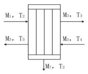
Fig. 2. Evaporator inlet and outlet model diagram.
