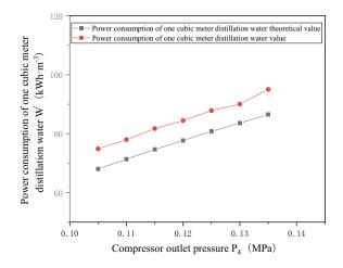
Fig. 9. Change of power consumption for production of 1 m<sup>3</sup> distilled water with change of discharge pressure.
