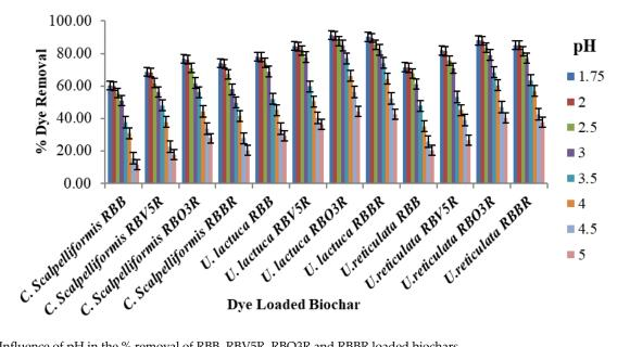
Fig. 3. Influence of pH in the % removal of RBB, RBV5R, RBO3R and RBBR loaded biochars.
