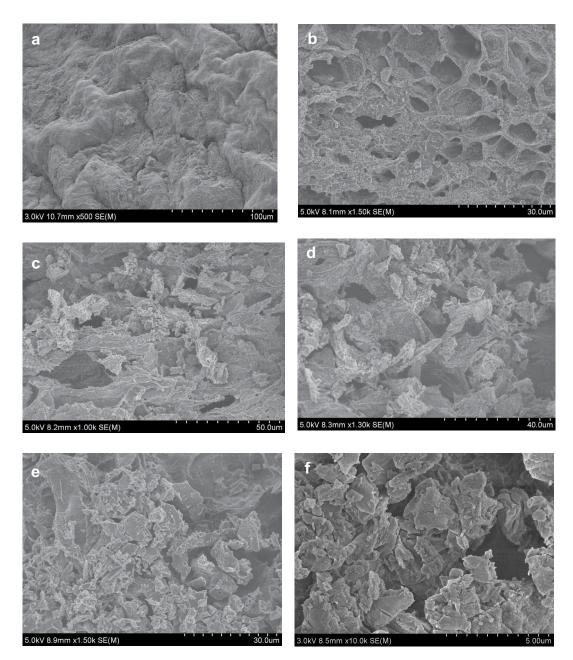
Fig. 9. Scanning electron micrographs of *C. scalpelliformis* (a), *C. scalpelliformis* derived biochar (b), RBB loaded biochar (c), RBV5R loaded biochar (d), RBO3R loaded biochar(e) and RBBR loaded biochar (f) [43].
