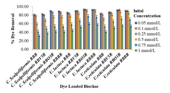
Fig. 5. Influence of initial concentration on the % removal of RBB, RBV5R, RBO3R and RBBR loaded biochars.
