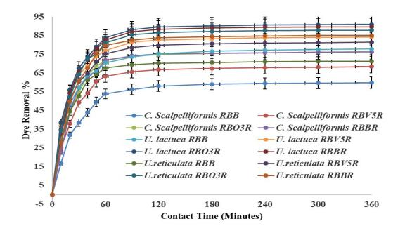
Fig. 6. Influence of contact time on the % removal of RBB, RBV5R, RBO3R and RBBR loaded biochars.
