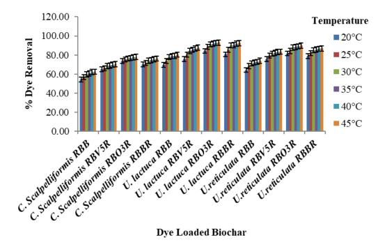
Fig. 4. Influence of temperature in the % removal of RBB, RBV5R, RBO3R and RBBR loaded biochars.
