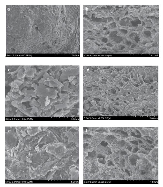
Fig. 8. Scanning electron micrographs of *U. reticulata* (a), *U. reticulata* derived biochar (b), RBB loaded biochar (c), RBV5R loaded biochar (d), RBO3R loaded biochar (e) and RBBR loaded biochar (f) [43].
