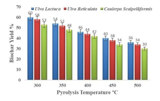
Fig. 1. Impact of pyrolysis temperature on the biochar yield for three green seaweed biomasses.
