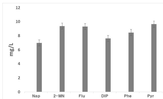
Fig. 2. Analysis of PAHs by the concentration of initial concentration test solution using GC-MS (naphthalene, 2-methylnaphthalene, fluorene, dibenzothiophene, phenanthrene, pyrene).
