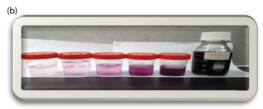
Figs. 2a and b. Picture of MB and arsenazo III dye after degradation at various times.
