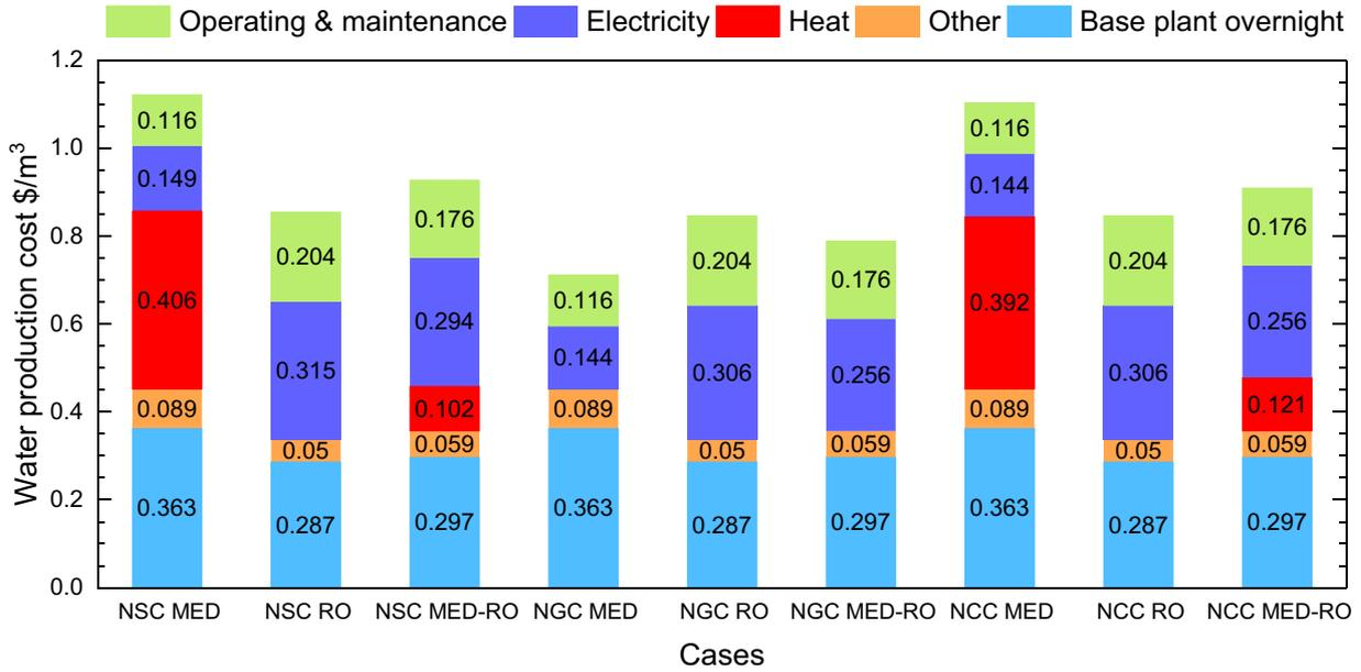
Fig. 5. Comparison of freshwater costs produced by various NPPs.
