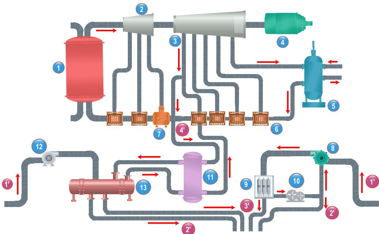
Fig. 4. Schematic drawing of NPP integrated with the hybrid desalination plant. Equipment: (1) steam generator, (2) high-pressure turbine, (3) low-pressure turbine, (4) generator, (5) condenser, (6) preheater, (7) deaerator, (8) high-pressure pump, (9) RO desalination plant, (10) energy recovery system, (11) intermediate heat exchanger, (12) feedwater pump, (13) MED desalination unit. Pipelines: (1') feedwater, (2') brine, (3') product water, and (4') hot steam.
