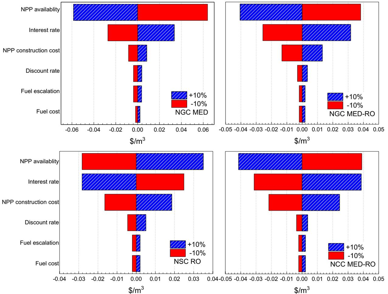
Fig. 6. Sensitivity analysis of different nuclear desalination scenarios.
