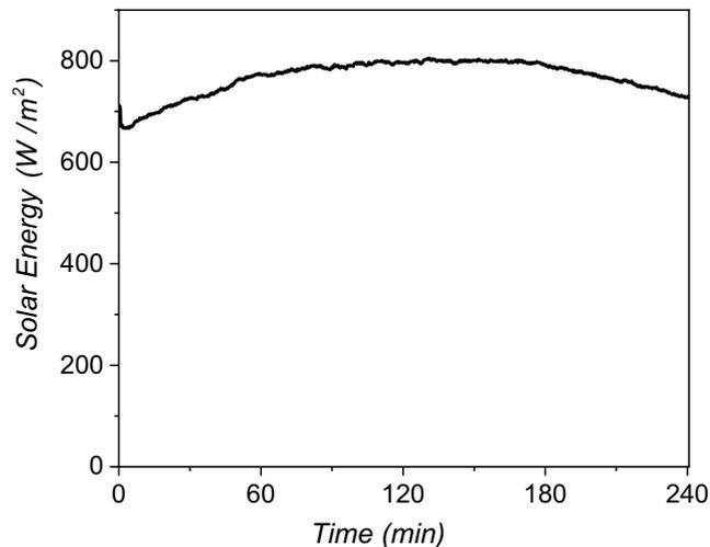
Fig. S3. Monitored solar energy in desalination of actual seawater using natural sunlight.
