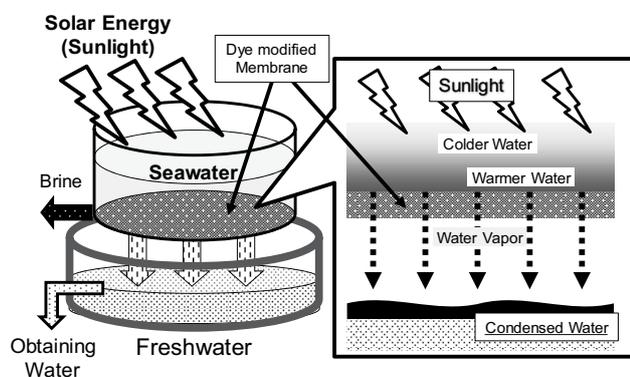
Fig. 1. A schematic diagram of solar desalination of seawater by membrane permeation with dye modified membrane using sunlight.
