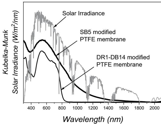
Fig. 5. Diffuse reflectance UV-vis-NIR spectra of DR1-DB14 doubly modified PTFE membrane and SB5 modified one (diameter: 47 mm). Kubelka-Munk functions are plotted against wavelength. Solar irradiance spectrum (Air Mass 1.5: Global tilt  $W/m^2/nm$ ) is also overlaid with adjusted vertical scale.
