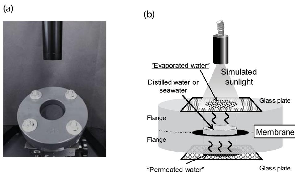
Fig. 3. (a) Image of the membrane permeation experiment using SB5 modified PTFE membrane sandwiched between two flanges (a slip-on type; in one flange, outer diameter: 115 mm, inner diameter: 42 mm, thickness: 14 mm). The distance from the lamp bottom to the membrane was about 225 mm. and (b) Schematic diagram of the membrane permeation experiment using flange system.
