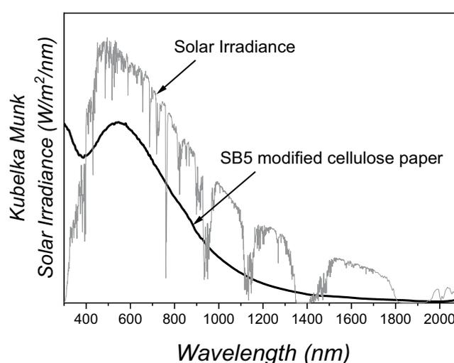
Fig. 7. Diffuse reflectance UV-vis-NIR spectrum of SB5 modified cellulose membrane (Kubelka-Munk function is plotted against wavelength). Solar irradiance spectrum is also overlaid with adjusted vertical scale.
