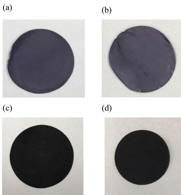
Fig. 4. Images of (a) DR1–DB14 doubly modified PTFE membrane (diameter: 47 mm), (b) SB5 modified PTFE membrane (diameter: 47 mm), (c) SB5 modified PTFE membrane (diameter: 55 mm), and (d) SB5 modified cellulose membrane (diameter: 40 mm). The scales of the images were adjusted.
