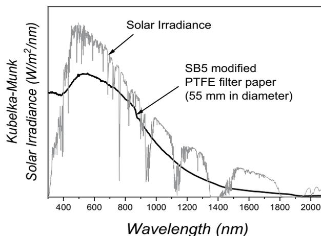
Fig. S2. Diffuse reflectance UV-vis-NIR spectrum of an SB5 modified PTFE membrane prepared from PTFE filter paper (diameter: 55 mm).
