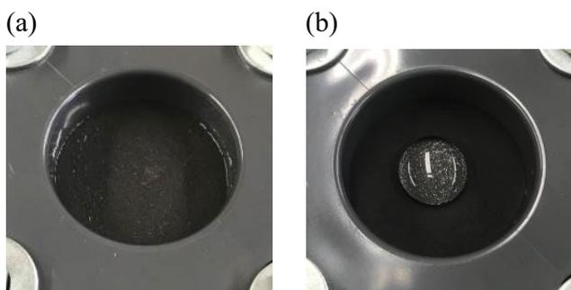
Fig. 6. States of distilled water on SB5 modified PTFE membrane. (a) 3 mL and (b) 1.0 mL.
