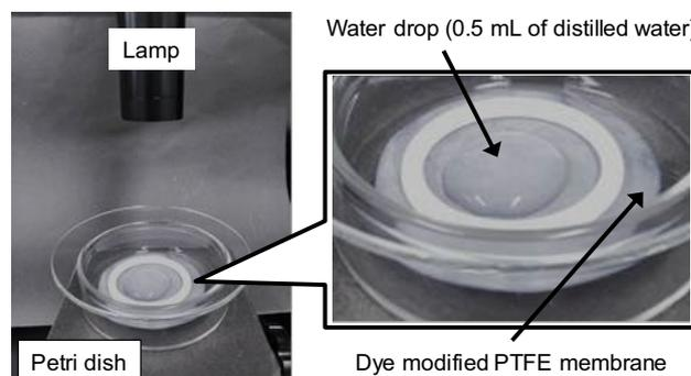
Fig. S1. Experimental apparatus of the membrane permeation by petri dish system.
