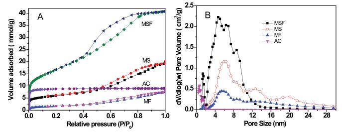
Fig. 1. (a) Nitrogen adsorption isotherms and (b) pore size distributions of MSF, MS, MF, and AC.
