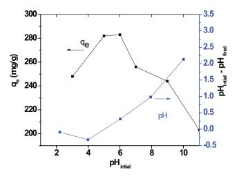
Fig. 4. Effect of pH on MSF adsorption capacity.
