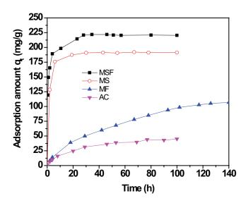
Fig. 3. Kinetic curves for CIP adsorption on the carbon adsorbents.
