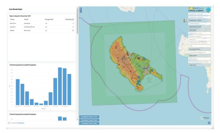
Fig. 8. Screenshot of the WebGIS application: drought alert status in the dashboard and information layer in the MapGIS for the outlook case (green: no alert, red: alert).
