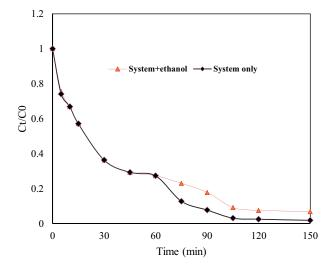
Fig. 8. Effect of scavenger (Fe<sub>3</sub>O<sub>4</sub> = 0.4 g/L; pH: 3; dye concentration: 20 mg/L; PS: 4 mM).
