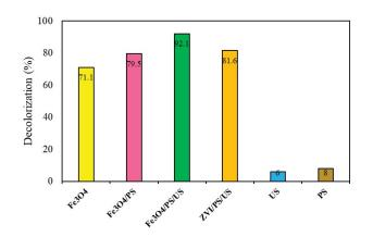
Fig. 9. Control of different process ( $Fe_3O_4 = 0.4 \text{ g/L}$ ; pH: 3; dye concentration: 20 mg/L; PS: 2 mM; ZVI: 0.4 g/L).
