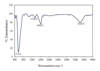
Fig. 2. FTIR of the synthesized Fe<sub>3</sub>O<sub>4</sub> for dye degradation.
