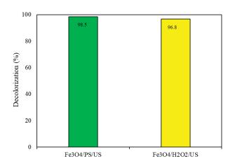
Fig. 6. Comparison between Fe<sub>3</sub>O<sub>4</sub>/PS/US and Fe<sub>3</sub>O<sub>4</sub>/H<sub>2</sub>O<sub>2</sub>/US (Fe<sub>3</sub>O<sub>4</sub> = 0.4 g/L; pH: 3; dye concentration: 20 mg/L; US: 200, PS, and H<sub>2</sub>O<sub>2</sub> = 4 mM).
