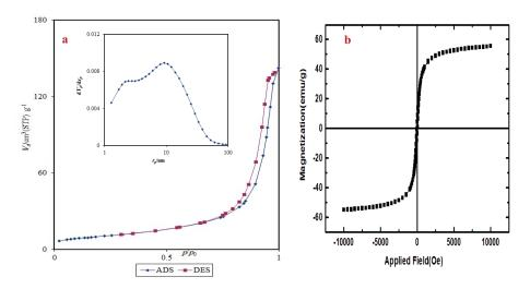
Fig. 3. (a) Adsorption/desorption isotherm of  $N_2$  on  $Fe_3O_4$  nanoparticles (insert: BJH pore size distribution) and (b) VSM image for  $Fe_3O_4$  nanoparticles for dye degradation.
