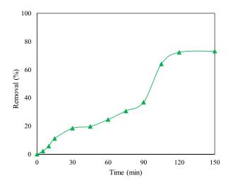
Fig. 11. TOC removal efficiencies by  $Fe_3O_4/US/PS$  process ( $Fe_3O_4 = 0.4 \text{ g/L}$ ; pH: 3; dye concentration: 20 mg/L; PS: 4 mM).
