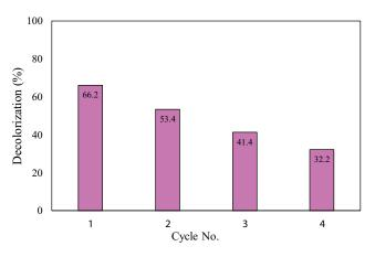
Fig. 10. Recovery (Fe<sub>3</sub>O<sub>4</sub> = 0.4 g/L; pH: 3; dye concentration: 20 mg/L; PS: 4 mM).
