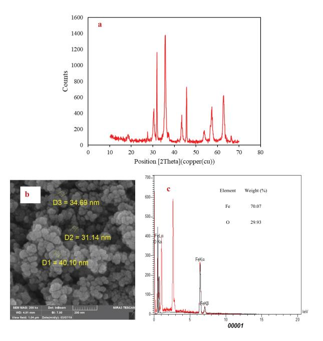
Fig. 1. (a) XRD pattern, (b) FE-SEM analysis, and (c) EDS of synthesized magnetic  $Fe_3O_4$  nanoparticle.
