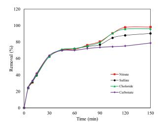
Fig. 7. Effect of various anion competition concentration (Fe<sub>3</sub>O<sub>4</sub> = 0.4g/L; pH: 3; dye concentration: 20 mg/L; US: 200; PS: 4 mM).
