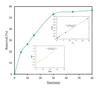
Fig. 4. Results of adsorption studies in removal of SSY (pH: 5; dye concentration: 30 mg/L;  $Fe_3O_4 = 0.4$  g/L).
