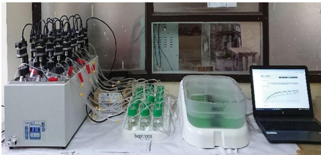
Fig. 3. Automated methane potential test system II (AMPTS II) experimental setup.
