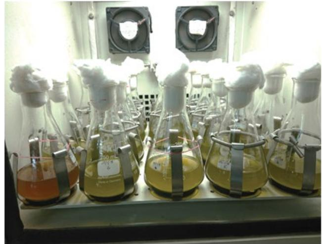
Fig. 1. Batch scale studies with shake flask experiments of different F/M ratios.
