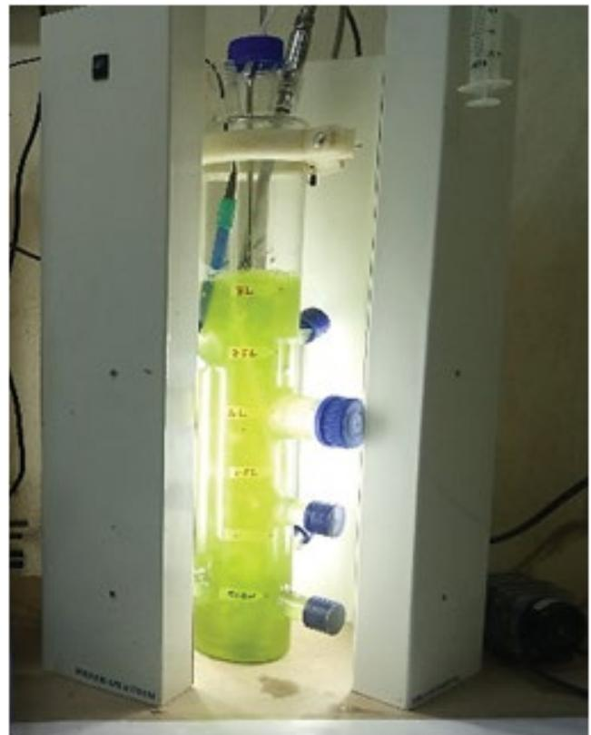
Fig. 2. Batch scale studies in a tubular photobioreactor with the optimized F/M Ratio.
