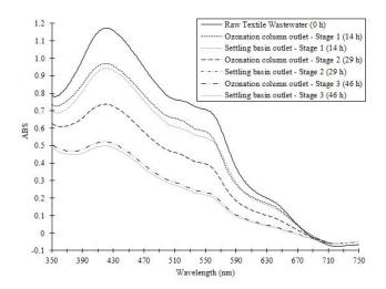
Fig. 3. Spectral scan of textile wastewater before and after the experimental stages 1 (O<sub>3</sub>: 13.6 mg/L; EC: 15.8 A), 2 (O<sub>3</sub>: 13.6 mg/L; EC: 22.1 A) and 3 (O<sub>3</sub>: 13.6 mg/L; EC: 28.5 A).
