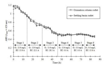
Fig. 2. Kinetics of color removal during different experimental stages.
