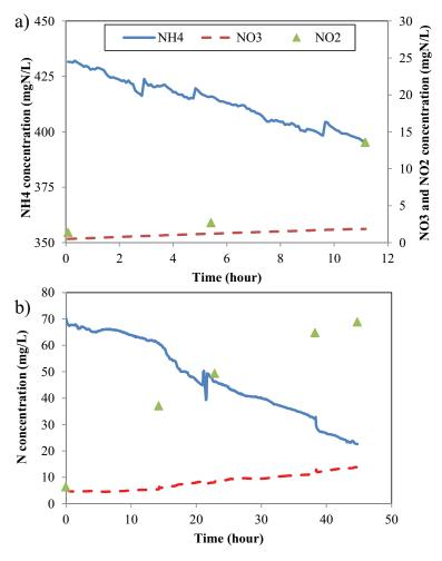
Fig. 7. Change of NH<sub>4</sub><sup>+</sup>-N, NO<sub>3</sub><sup>-</sup>-N and NO<sub>7</sub><sup>-</sup>-N concentrations of biofilm system under sidestream and mainstream conditions.
