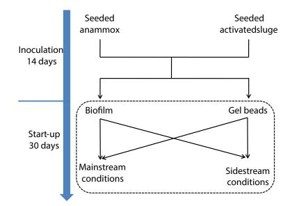
Fig. 1. Experimental procedure of inoculation and start-up periods.
