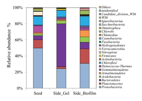
Fig. 4. Microbial community composition at phylum level in seeded sludge (Seed), gel bead (Side\_Gel) and biofilm (Side\_Biofilm) under sidestream conditions (relative abundance less than 0.1% is included as others).
