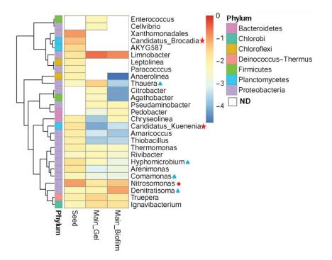
Fig. 3. Heat map of genera in seeded sludge (Seed), gel bead (Main\_Gel) and biofilm (Main\_Biofilm) cultured under mainstream conditions. Values plotted are the relative abundance after log10 transformed. Anammox bacteria: red  $\star$ ; Ammonia-oxidizing bacteria: red  $\bullet$ ; Denitrifier: blue  $\blacktriangle$ .
