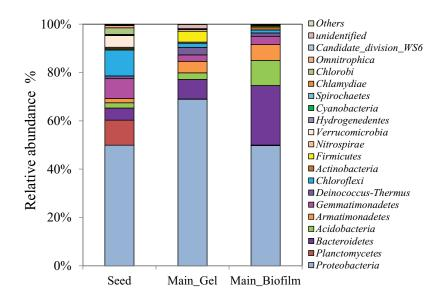
Fig. 2. Microbial community composition at phylum level in seeded sludge (Seed), gel bead (Main\_Gel) and biofilm (Main\_Biofilm) under mainstream conditions (relative abundance less than 0.1% is included as others).
