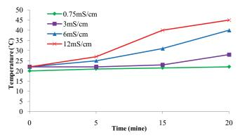
Fig. 2. Effect of duration and solution conductivity on the solution temperature.
