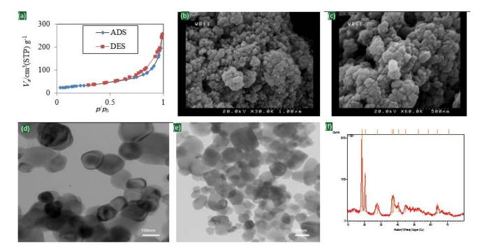
Fig. 6. BET plots of nitrogen adsorption–desorption isotherms (a), FE-SEM image at different magnifications (b and c), TEM Image at different magnifications (d and e), and X-ray diffraction patterns (f) of the Alum nanocrystallites.
