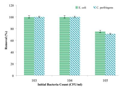
Fig. 4. Effect of initial bacteria count on removal efficiency of *E. coli* and *C. perfringens* (initial bacteria count:  $10^3$ – $10^5$  CFU/mL, initial pH: 7, reaction time: 25 min, CD: 33.3 A/m<sup>2</sup>, IED: 2 cm, and conductivity: 0.75 mS/cm). The mean value obtained from two separate experiments are demonstrated in data shown in the figure. Three replicates were carried out for every condition and the error bar is representative of standard deviation.
