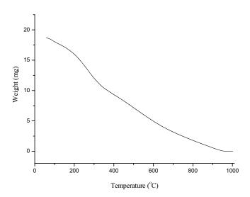
Fig. 3. TGA curve of PGP-1N H<sub>2</sub>SO<sub>4</sub>.
