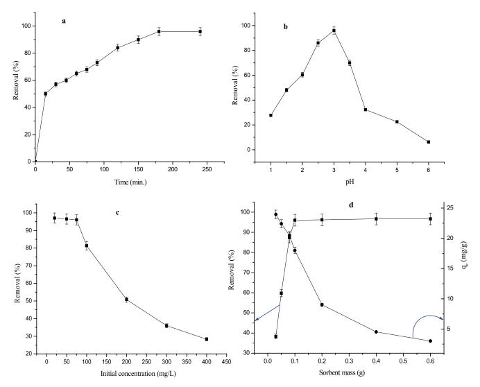
Fig. 5. Effect of some operational parameters on the removal of Cr(VI) by PGP-1N  $H_2SO_4$  (a) time, (b) pH, (c) initial concentration, and (d) sorbent mass.
