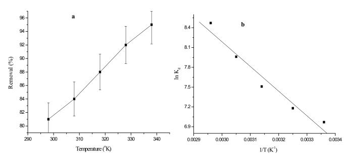
Fig. 9. Effect of reaction temperature on (a) removal (%) and (b) Van't Hoff plots for the removal of Cr(VI) by using PGP-1N H<sub>2</sub>SO<sub>4</sub> at an agitating rate, 250 rpm; initial metal concentration, 100 mg/L; contact time, 180 min; volume, 25 mL; weight, 0.1 g; pH, 3.
