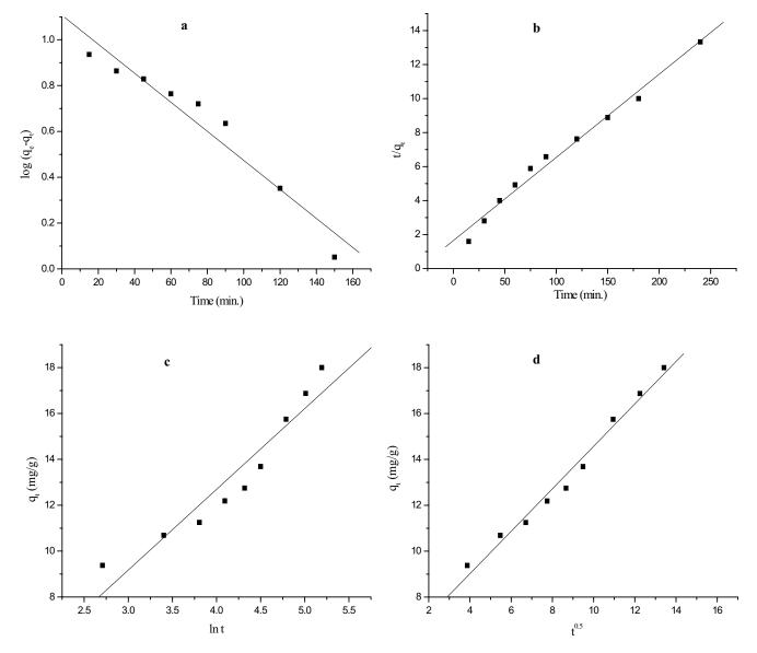
Fig. 7. Kinetics of Cr(VI) adsorption onto PGP-1N  $H_2SO_4$  (a) pseudo-first-order model, (b) pseudo-second-order model, (c) Elovich model, and (d) intraparticle diffusion at initial Cr(VI) concentration 75 mg/L, pH = 3.0, and 25°C ± 1°C.
