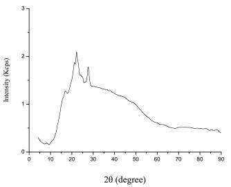
Fig. 4. XRD pattern of PGP-1N H<sub>2</sub>SO<sub>4</sub>.
