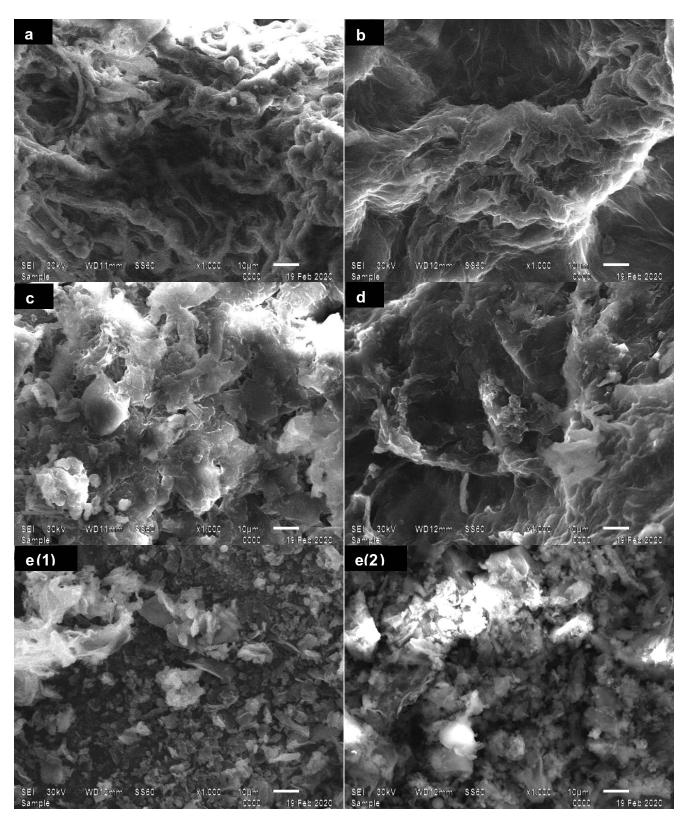
Fig. 1. SEM micrographs of (a) untreated-PGP, (b) PGP-1N HNO<sub>3</sub>, (c) PGP-1N HCl, (d) PGP-1N NaOH, (e) [(1) PGP-1N  $H_2SO_4$  and (2) Cr-sorbed PGP-1N  $H_2SO_4$ ] magnitude of 1,000×.
