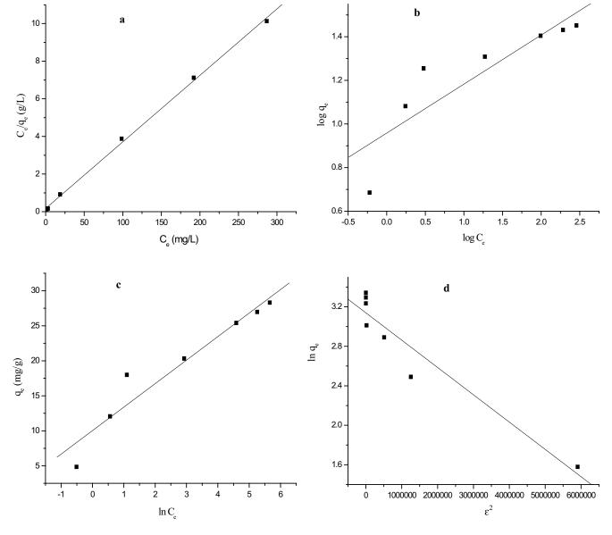
Fig. 8. Linearized form of (a) Langmuir, (b) Freundlich, (c) Temkin, and (d) Dubinin–Radushkevich isotherm models for the adsorption of Cr(VI) onto PGP-1N H<sub>2</sub>SO<sub>4</sub> sample at 25°C ± 1°C.
