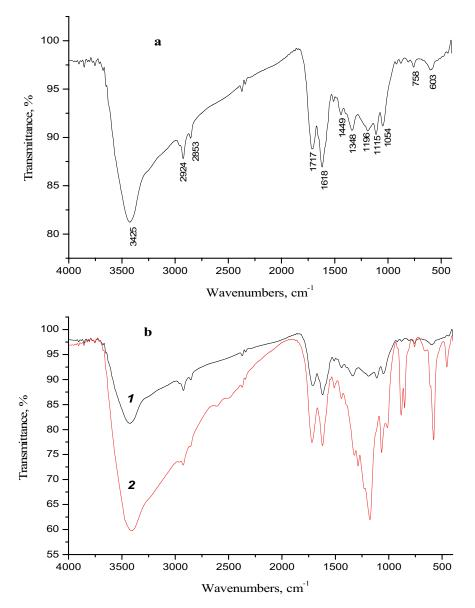
Fig. 2. FT-IR spectrum of (a) PGP-1N H<sub>2</sub>SO<sub>4</sub> sample and (b) [(1) unloaded PGP-1N H<sub>2</sub>SO<sub>4</sub> and (2) Cr-sorbed PGP-1N H<sub>2</sub>SO<sub>4</sub>].
