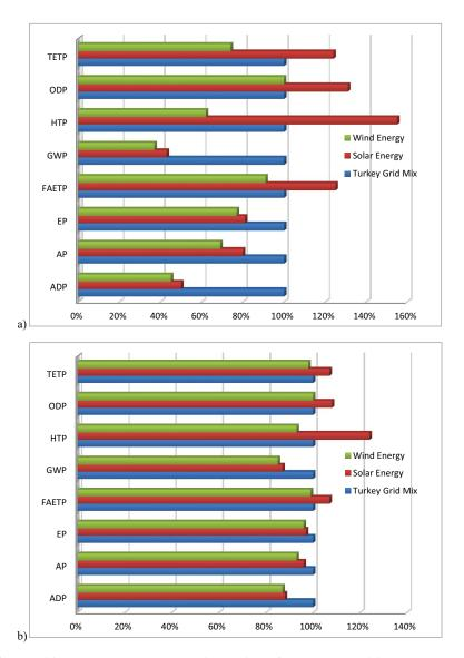
Fig. 6. Relative impact of renewable energy sources compared to grid mix for (a) case 1 and (b) case 2.
