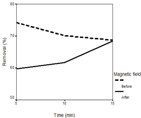
Fig. 3. Effects of the magnetic field on the arsenic removal efficiency vs. contact time based on iron filings dosage of 2.5 g/L.
