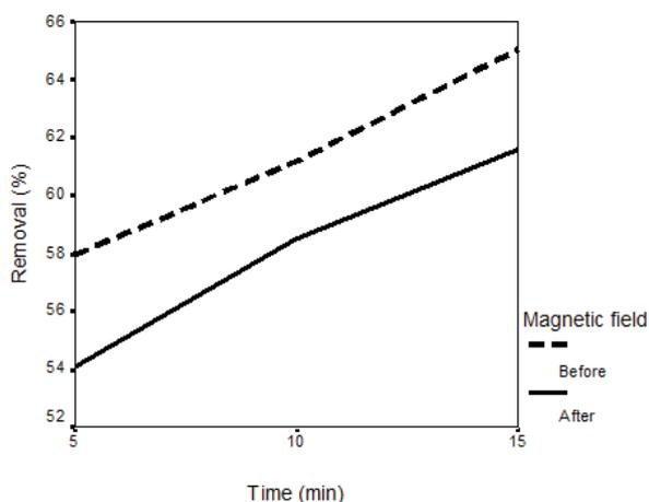
Fig. 6. Effects of the magnetic field on the arsenic removal efficiency vs. contact time based on the initial arsenic concentration of 2 mg/L.
