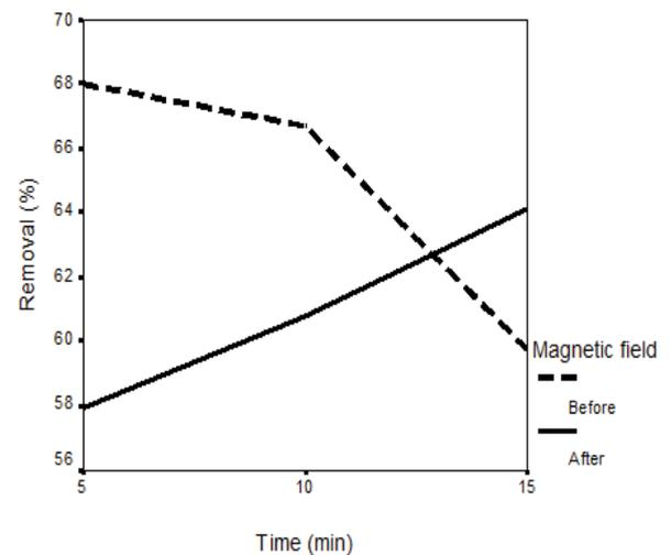
Fig. 5. Effects of the magnetic field on the arsenic removal efficiency vs. contact time based on the initial arsenic concentration of 0.5 mg/L.
