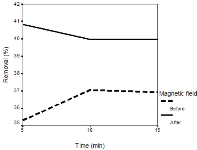
Fig. 2. Effects of the magnetic field on the arsenic removal efficiency vs. contact time based on iron filings dosage of 0 g/L.
