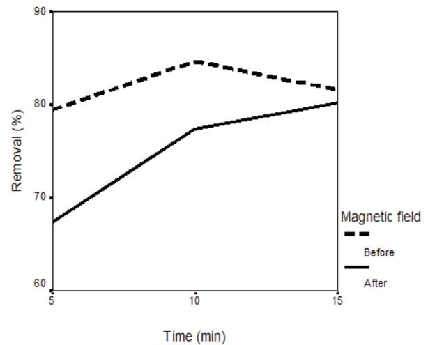
Fig. 4. Effects of the magnetic field on the arsenic removal efficiency vs. contact time based on iron filings dosage of 5 g/L.
