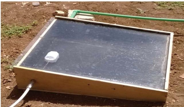
Fig. 3. Basin type solar still used in the experiment.
