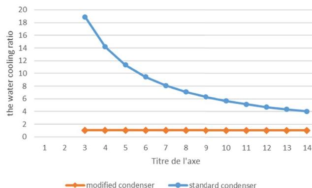
Fig. 10. Variation cooling water ratio with the number of effects.
