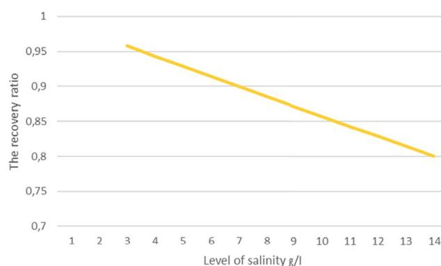
Fig. 11. Recovery ratio variation regarding the level of water salinity.
