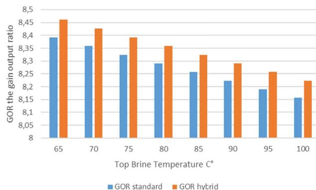
Fig. 9. Gain output ratio variation regarding the top brine temperature for both configurations.
