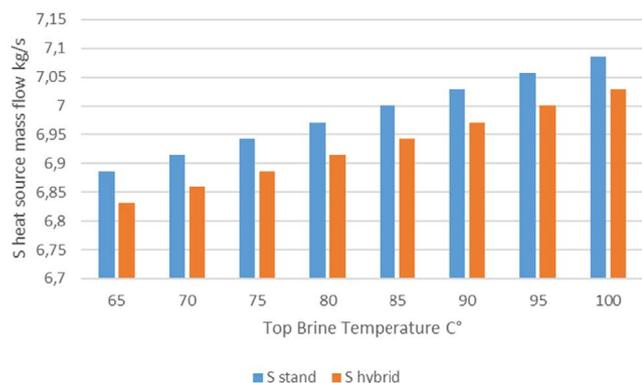
Fig. 8. Heat source mass flow variation regarding the top brine temperature for both configurations.
