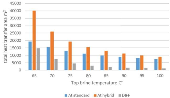
Fig. 5. Variation of total heat transfer area regarding the top brine temperature for both configurations.
