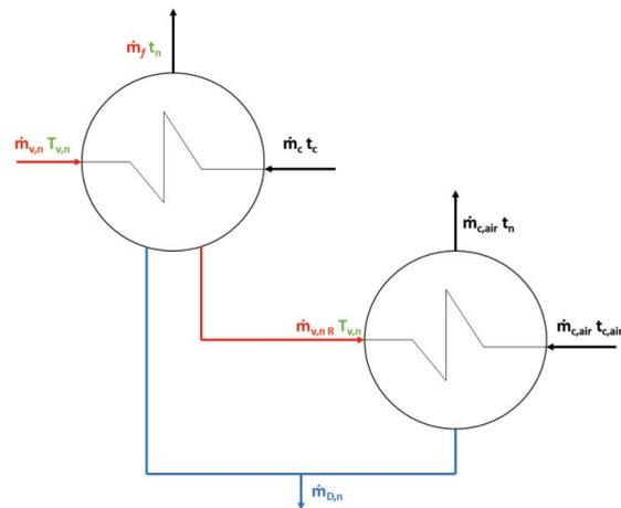
Fig. 3. Hybrid condenser.
