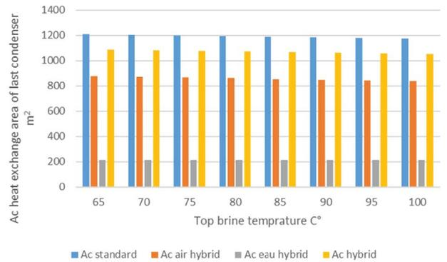
Fig. 6. Variation of the heat exchange area of the last condenser for both configurations.
