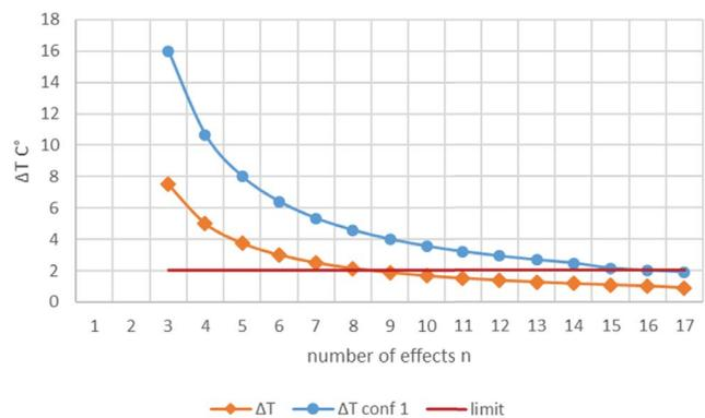
Fig. 4. Limit of the effects number on the MED water condenser configuration and the MED-hybrid condenser.
