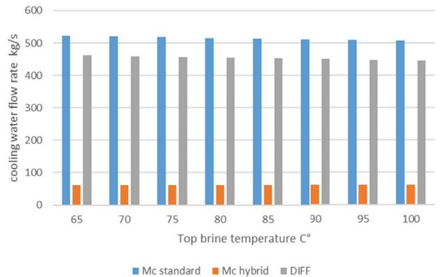
Fig. 7. Variation of the cooling water mass flow for both configurations.
