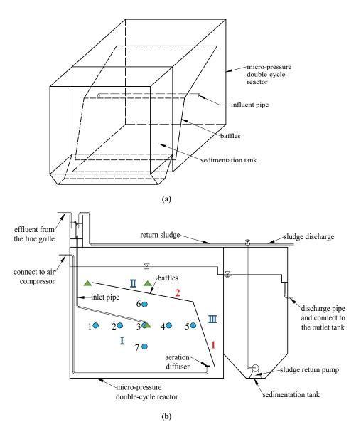
Fig. 3. (a) Three-dimensional schematic diagram of pilot test device and (b) schematic diagram of technological process and distribution of test points of pilot test device. *Note:*
