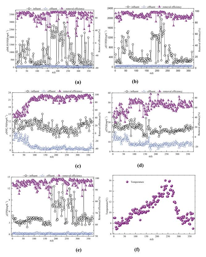
Fig. 5. (a) SS removal effect of pilot test device, (b) COD removal effect of pilot test device, (c)  $NH_4^*$ -N removal effect of pilot test device, (d) TN removal effect of the pilot test device, (e) TP removal effect of the pilot test device, and (f) influent temperature change during the test.
