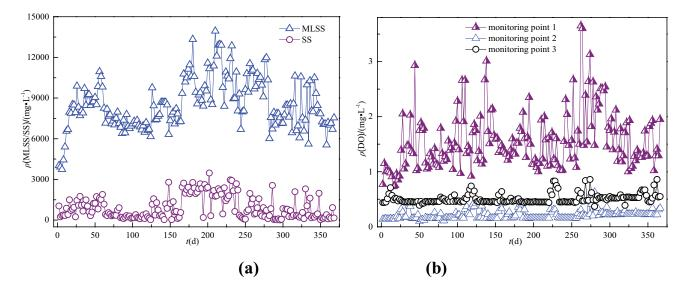
Fig. 6. (a) Changes in average MLSS concentration in the reactor and changes in SS concentration in the influent during the test and (b) changes in DO during the test period at three DO monitoring points.
