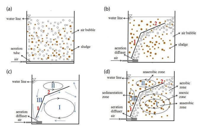
Fig. 1. (a) Schematic diagram of traditional biological aeration tank, (b) schematic diagram of MPDR biological aeration tank, (c) schematic diagram of MPDR mixed liquid flow distribution in ideal state, and (d) schematic diagram of MPDR different dissolved oxygen zones in ideal state.
