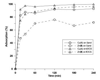
Fig. 2. Adsorption of Cu(II) and Zn(II) on sand and IOCS with respect to time.
