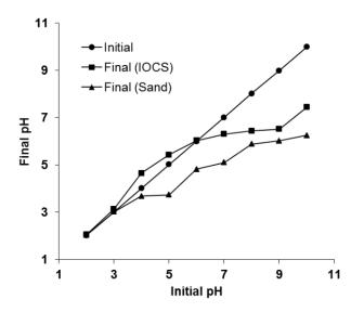
Fig. 1. Determination of  $\text{pH}_{\text{PZC}}$  for sand and IOCS by the salt addition method.
