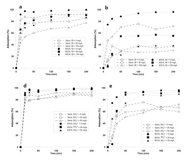
Fig. 4. Adsorption kinetics of heavy metals on sand and IOCS with varying concentrations of chloride and sulfate ions (adsorbent dose = 5 g/100 mL): (a) Cu(II) with Cl<sup>-</sup>, (b) Zn(II) with Cl<sup>-</sup>, (c) Cu(II) with SO<sub>4</sub><sup>2-</sup>, and (d) Zn(II) with SO<sub>4</sub><sup>2-</sup>.
