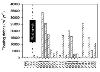
Fig. 4. Yearly distribution of floating debris in Daecheong Reservoir from 1996 to 2020.
