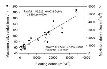
Fig. 5. Scatter plot showed a simple linear regression between floating debris and maximum daily rainfall and the debris and maximum inflow in Daecheong Reservoir (number of data = 26).
