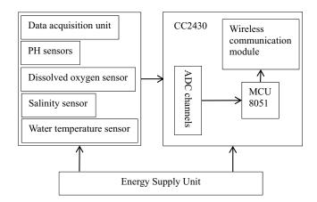
Fig. 2. Structure design of sensor at acquisition end.
