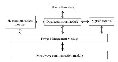
Fig. 3. Structure design of monitoring terminal.
