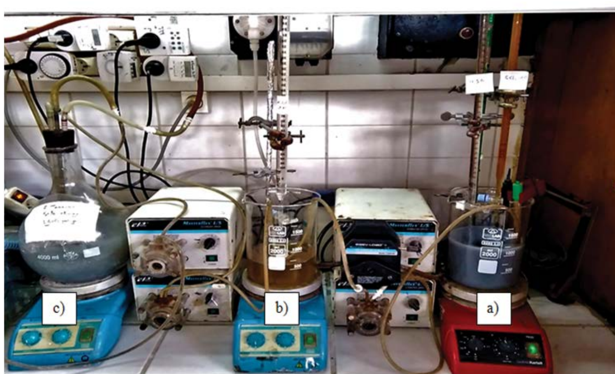
Fig. 1. Combination of precipitation and SBR systems for treatment of tannery effluent in the laboratory. Beaker for (a) chemical process, (b) pH neutralization, and (c) SBR process.
