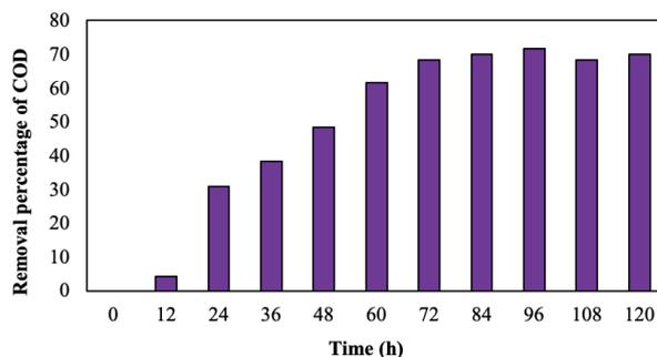
Fig. 3. COD removal in a mixed drug solution containing CEF and RAN by activated sludge in an SBR; drug concentration of  $30 \text{ mg L}^{-1}$  each,  $\text{pH}_0 = 7.17$ ,  $\text{MLSS}_0 = 1,540 \text{ mg L}^{-1}$ ,  $\text{DO} = 2.5 \text{ mg L}^{-1}$ .
