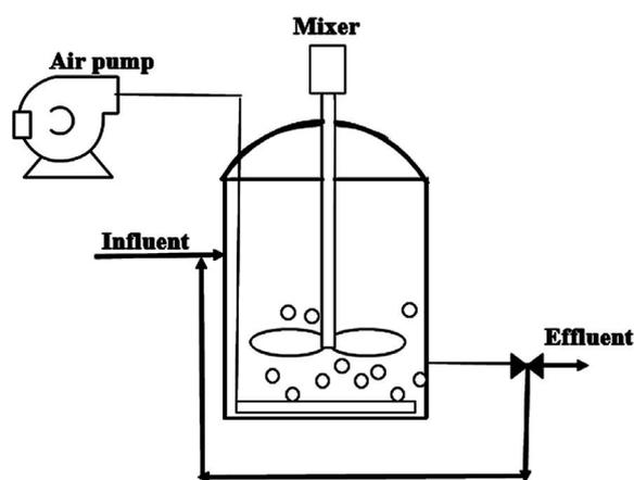
Fig. 1. Schematic of the laboratory SBR for the simultaneous removal of CEF and RAN by activated sludge.
