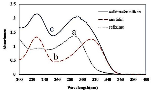
Fig. 2. The absorbance spectra of aqueous (a) CEF solution (30 mg L<sup>-1</sup>), (b) RAN solution (30 mg L<sup>-1</sup>), and (c) mixture of CEF and RAN (30 mg L<sup>-1</sup> each).
