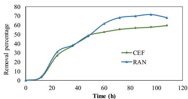
Fig. 4. The removal percentage of CEF and RAN via activated sludge in an SBR; initial concentration of each drug =  $30 \text{ mg L}^{-1}$ ,  $\text{pH}_0 = 7.17$ ,  $\text{MLSS}_0 = 1,540 \text{ mg L}^{-1}$ ,  $\text{DO} = 2.5 \text{ mg L}^{-1}$ .
