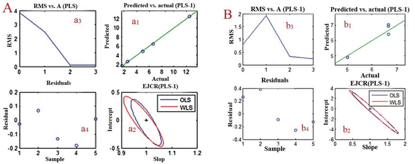
Fig. 5. Graphical form of RMSEP validation data for the monitoring of simultaneous removal of RAN (A) and CEF (B) ( $30 \text{ mg L}^{-1}$  each) by activated sludge in an SBR.
