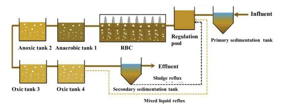
Fig. 1. Diagram of treatment units and processes used in the WWTP system.
