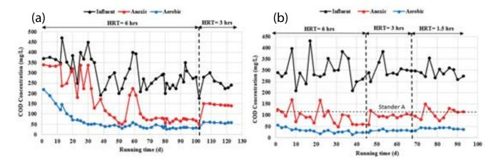
Fig. 5. COD concentration vs. time for (a) non-coated cosmoball and (b) coated cosmoball.
