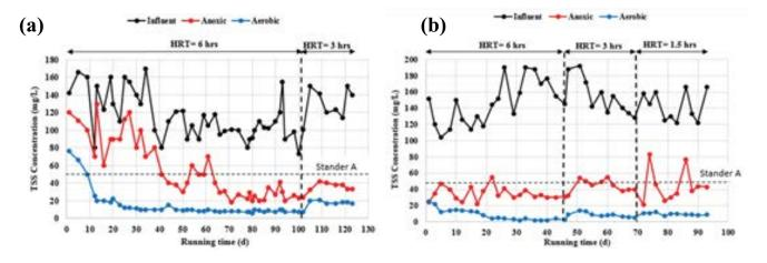
Fig. 6. TSS concentration vs. time for (a) non-coated cosmoball and (b) coated cosmoball.
