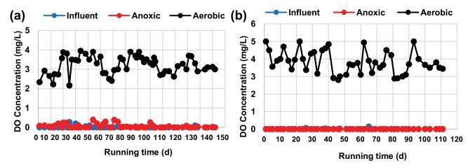
Fig. 12. DO concentration for (a) non-coated and (b) coated media.
