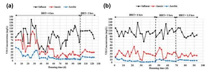
Fig. 7. VSS concentration vs. time for (a) non-coated cosmoball and (b) coated cosmoball.
