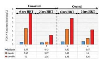
Fig. 10. Nitrate concentration under feeding, anoxic and aerobic conditions when coated and non-coated media were used at HRT of 6 and 3 h.
