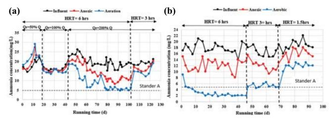
Fig. 8. Ammonia nitrogen concentration vs. time for (a) non-coated cosmoball and (b) for coated cosmoball.
