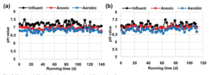
Fig. 13. Variation of pH with time for (a) non-coated and (b) coated media.
