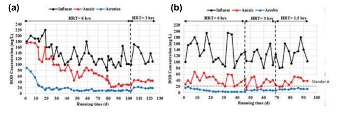
Fig. 4. BOD<sub>5</sub> concentration vs. time for (a) non-coated cosmoball and (b) coated cosmoball.
