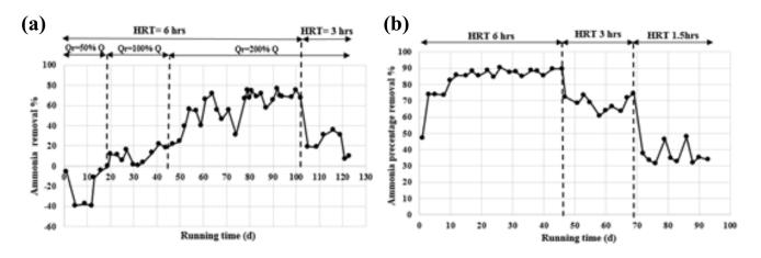
Fig. 9. Ammonia nitrogen removal by (a) non-coated cosmoball and (b) coated cosmoball.
