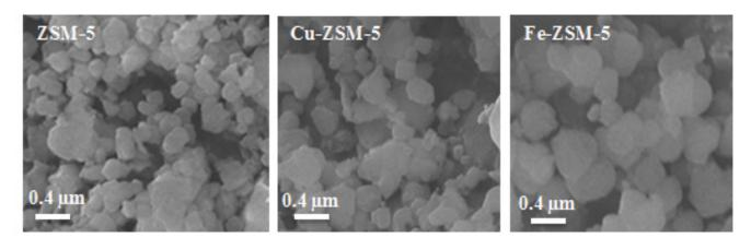
Fig. 3. SEM of different ZSM-5 catalysts.
