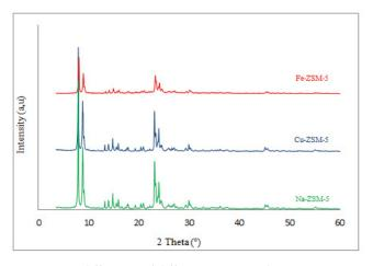
Fig. 1. X-ray diffraction of different ZSM-5 zeolites.
