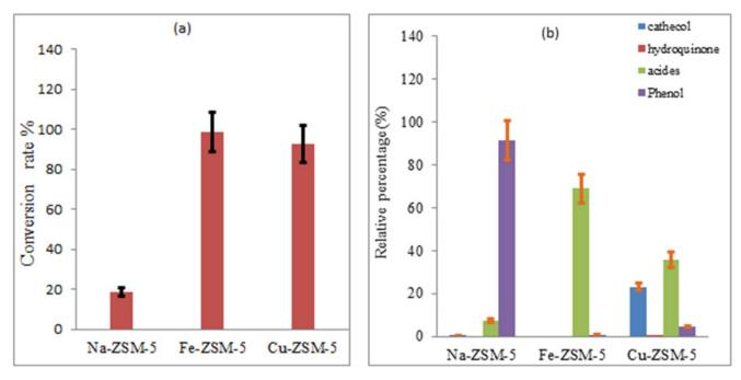
Fig. 4. (a) Conversion rate of phenol on ZSM-5 catalysts and (b) distribution of by-products by ZSM-5 catalysts. ( $t = 240 \text{ min}, T = 70^{\circ}\text{C}, C_{\text{Ph}} = 0.01 \text{ mol } \text{dm}^{-3}, C_{\text{H2O2}} = 0.10 \text{ mol } \text{dm}^{-3}, m_{\text{cat}} = 0.1 \text{ g } \text{dm}^{-3}, \text{pH} = 4.8$ ).
