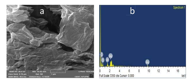
Fig. 3. (a) Morphological structure and (b) elemental composition of synthesized graphene oxide.
