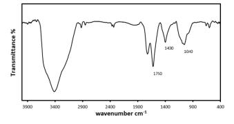
Fig. 4. FTIR spectra of synthesized graphene oxide (% transmittance as a function of inverse wavenumber).
