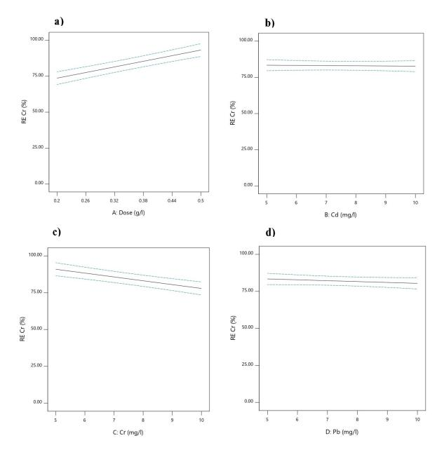
Fig. 9. Effect of (a) GO dosage, (b) cadmium concentration, (c) chromium concentration, and (d) lead concentration on to adsorption capacity of chromium.
