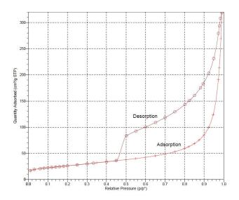
Fig. 5.  $N_2$  adsorption–desorption isotherm of synthesized graphene oxide ( $N_2$  adsorbed vs. relative pressure).
