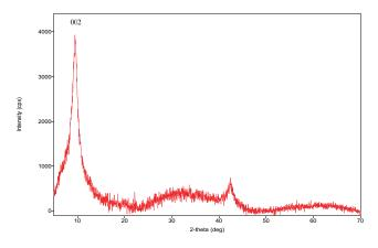
Fig. 2. XRD pattern of synthesized graphene oxide.
