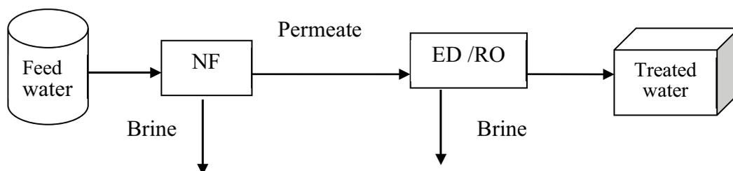
Fig. 4. Procedure of the NF-RO and NF-ED hybrid systems.
