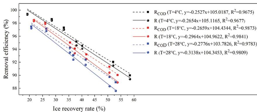
Fig. 9. Variations of salt and COD removal efficiencies with ice recovery rate using FGCM treatment under different ambient temperatures (salt organic wastewater samples, ambient temperature at  $28^\circ\text{C}$ ,  $18^\circ\text{C}$  and  $4^\circ\text{C}$ ).
