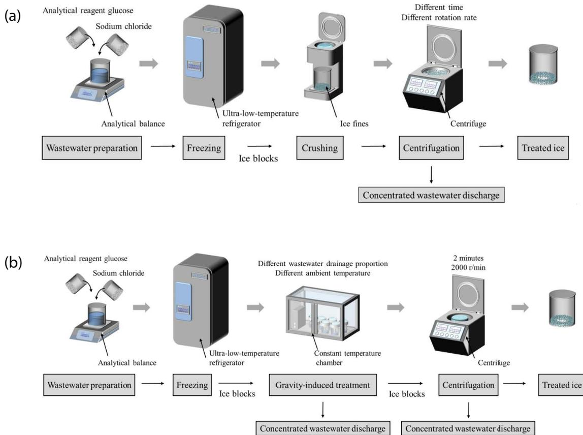
Fig. 1. Flow diagram of (a) FCM and (b) FGCM.
