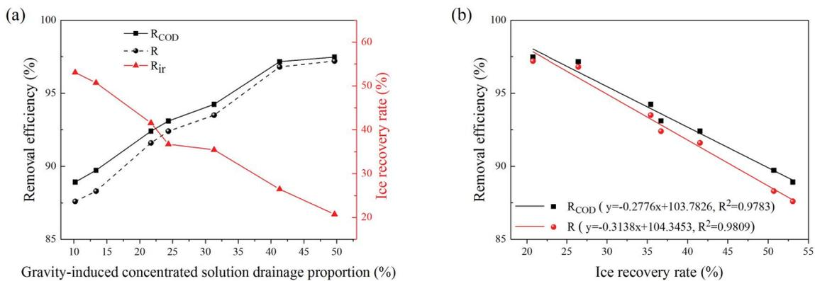
Fig. 7. Change of FGCM treatment effect under different gravity-induced concentrated wastewater drainage proportion (salt organic wastewater samples, ambient temperature at 28°C): (a) presents the variations of salt and COD removal efficiencies and ice recovery rate with gravity-induced concentrated wastewater drainage proportion and (b) presents the variations of salt and COD removal efficiencies with ice recovery rate.
