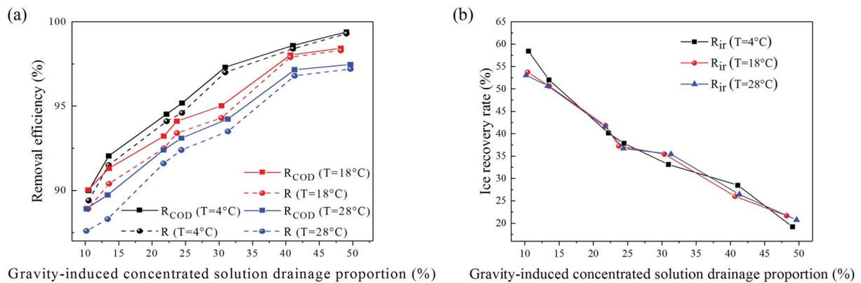
Fig. 8. Comparison of FGCM treatment effect under different ambient temperatures (salt organic wastewater samples, ambient temperature at  $28^\circ\text{C}$ ,  $18^\circ\text{C}$  and  $4^\circ\text{C}$ ): (a) presents the variations of salt and COD removal efficiencies with gravity-induced concentrated wastewater drainage proportion and (b) presents the variations of ice recovery rates with gravity-induced concentrated wastewater drainage proportion.
