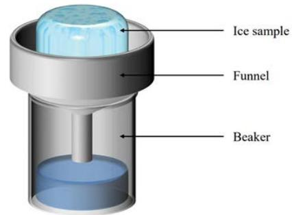
Fig. 3. Schematic of the gravity-induced ice melting process.
