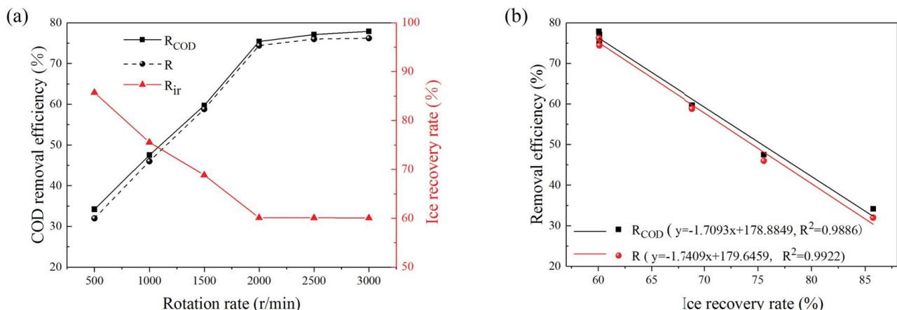
Fig. 6. Change of FCM treatment effect under different centrifuge rotation rate for salt organic wastewater samples: (a) presents the variations of salt and COD removal efficiencies and ice recovery rate with centrifuge rotation rate and (b) presents the variations of salt and COD removal efficiencies with ice recovery rate.
