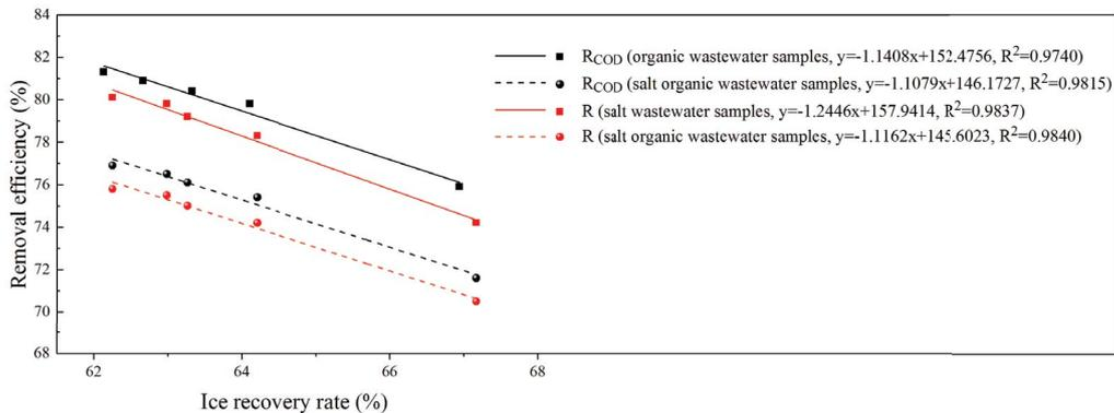
Fig. 5. Variations of salt and COD removal efficiencies with ice recovery rate using FCM treatment for three kinds of wastewater samples under different centrifugation duration.
