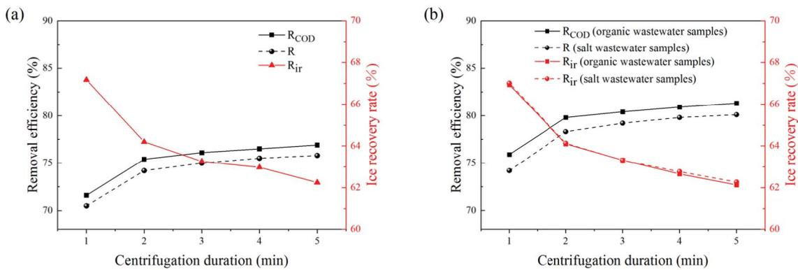
Fig. 4. Change of FCM treatment effect under different centrifugation duration: (a) presents the results with salt organic wastewater samples and (b) presents the results with organic wastewater samples and salt wastewater samples.
