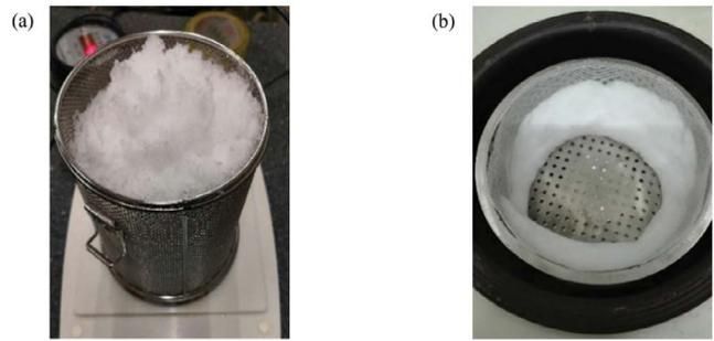
Fig. 2. (a) Crushed and (b) centrifuged ice sample.
