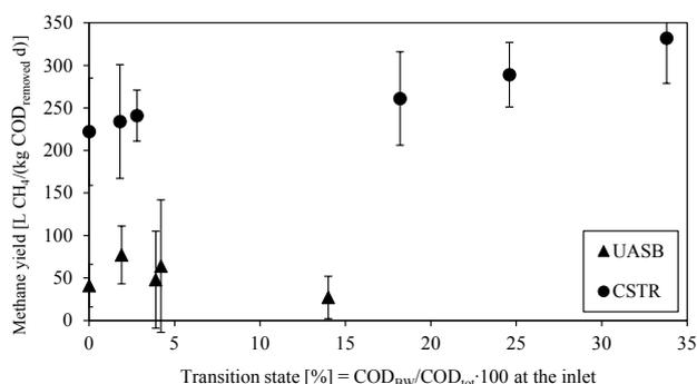
Fig. 3. Methane yield during different transition states of CSTR and UASB reactors.
