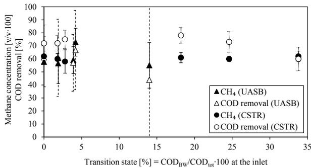
Fig. 2. Methane concentration in biogas and COD elimination during different transition states for CSTR (solid and empty circles) and UASB (solid and empty triangles) reactors. Bars indicate standard deviation of methane fraction, while dotted lines indicate standard deviation of COD elimination.
