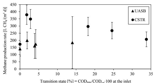
Fig. 4. Methane production rate during different transition states for CSTR and UASB reactors.
