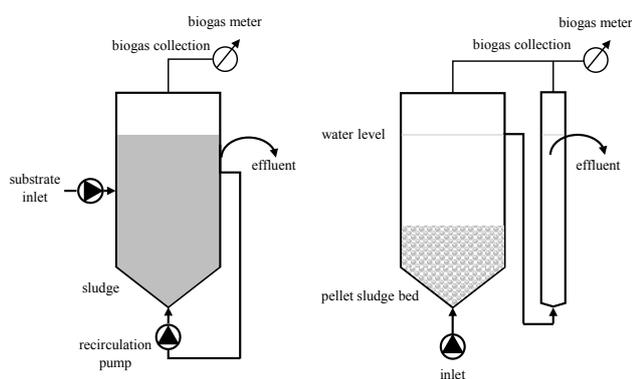
Fig. 1. Schematic setup for CSTR (left) and UASB (right) reactor; substrate storage tanks are not depicted.
