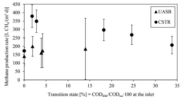
Fig. 4. Methane production rate during different transition states for CSTR and UASB reactors.
