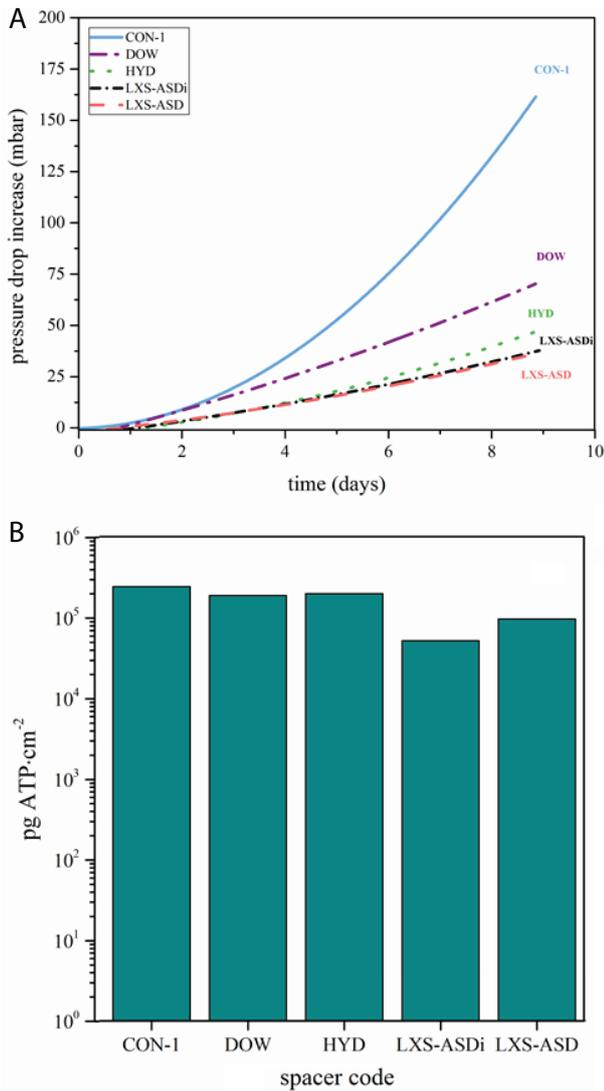
Fig. 1. (A) Pressure drop increase in time in MFSs containing one reference and four modified feed spacers at a constant feed flow rate and (B) accumulated viable biomass content (pg ATP.cm<sup>-2</sup>) for the short-term (9-d) biofouling study accelerated with nutrient dosage [20].
