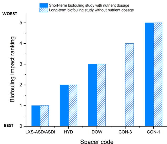
Fig. 3. Biofouling impact ranking of two reference and four modified feed spacers based on the 9-d short-term (with nutrient dosage) and 96-day long-term (without nutrient dosage) biofouling studies [20].
