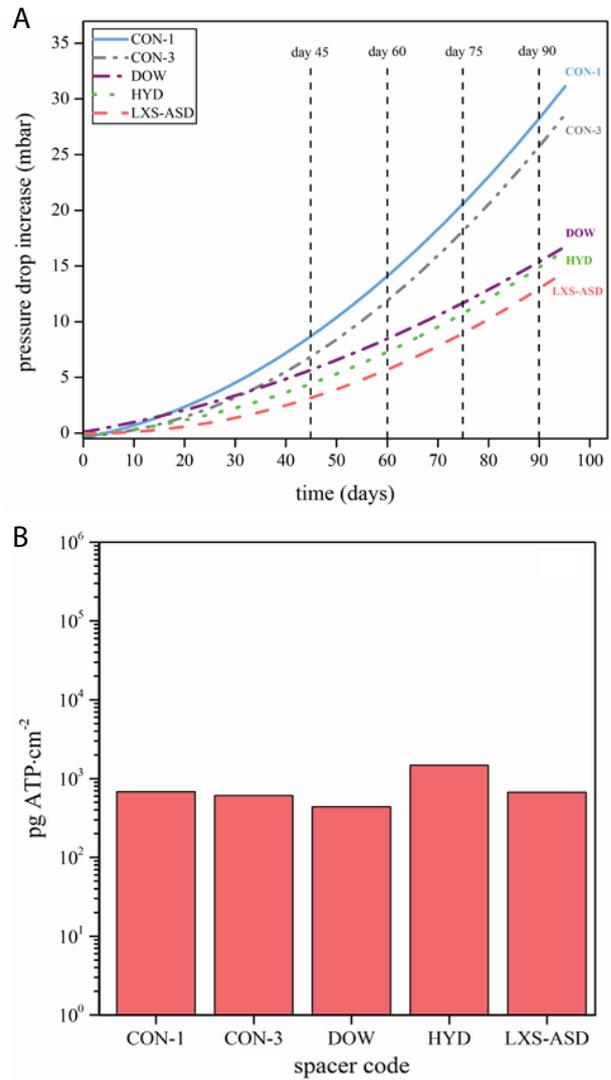
Fig. 2. (A) Pressure drop increase in time in MFSs containing two reference and three modified feed spacers at a constant feed flow rate and (B) accumulated viable biomass content (pg ATP.cm<sup>-2</sup>) during the long-term (96-d) biofouling study without nutrient dosage [20].
