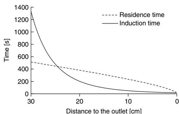
Fig. 7. Comparison of induction time and residence time for electro dialysis of solution no. 3.
