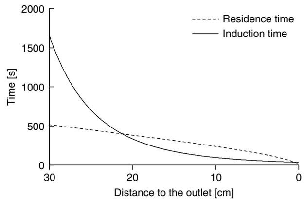
Fig. 5. Comparison of induction time and residence time for electro dialysis of solution no. 1.
