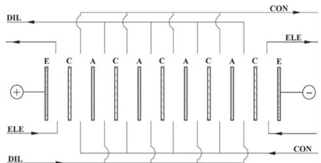
Fig. 2. The membrane stack configuration: C – cation-exchange membrane, A – anion-exchange membrane, E – platinum-coated titanium electrode, ELE – electrode rinse solution, CON – concentrate, DIL – diluate.
