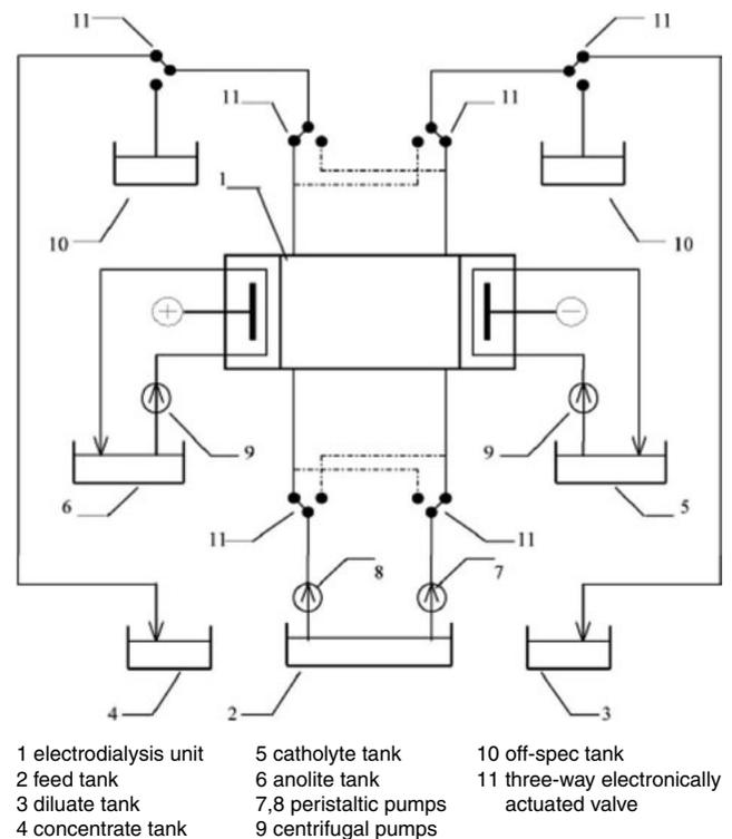
Fig. 1. Schematic diagram of EDR measuring equipment.
