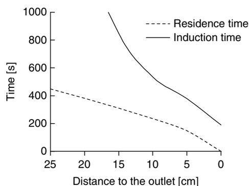
Fig. 9. Comparison of induction time and residence time for calcium bicarbonate solution.
