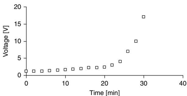
Fig. 3. Voltage drop across membrane stack during electrodi-lysis of solution no. 1.
