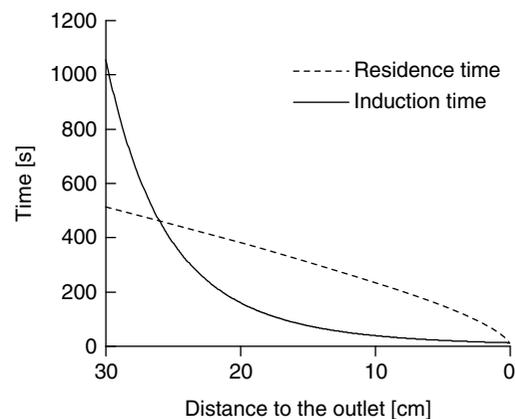
Fig. 6. Comparison of induction time and residence time for electro dialysis of solution no. 2.
