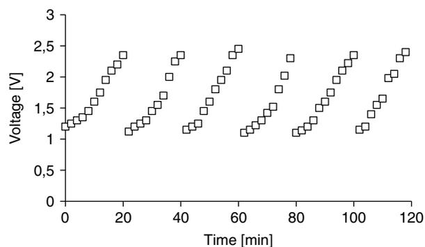
Fig. 4. Voltage drop across membrane stack during electrodi-lysis reversal of solution no. 1.
