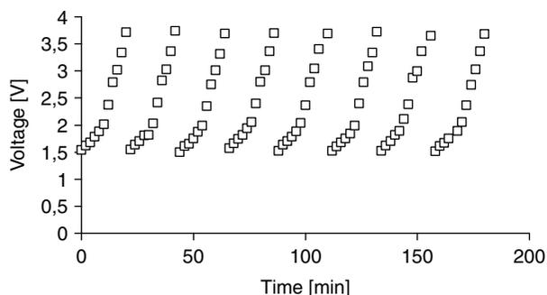
Fig. 8. EDR voltage drop across membrane stack over time, calcium carbonate feed at current density 23 A m<sup>-2</sup> and diluate recovery 94.6%.
