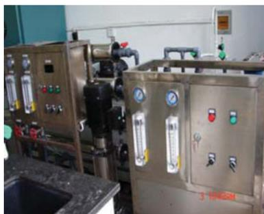
Fig. 3. Combined membranes treatment system.
