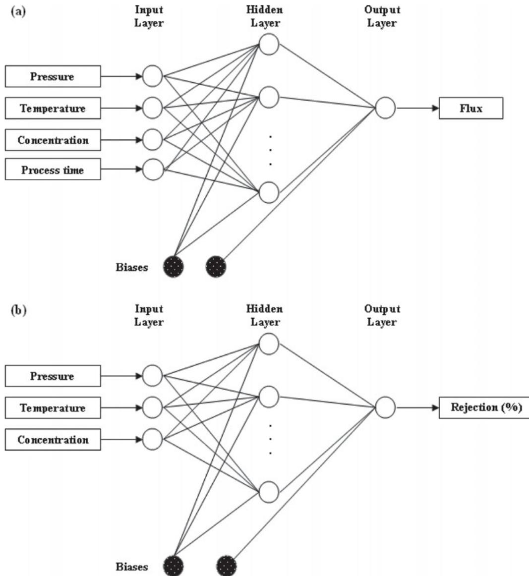
Fig. 1. Schematic of multi-layer feed forward neural network architectures with one hidden layer used for prediction of (a) permeate flux, and (b) ionic compounds rejections.
