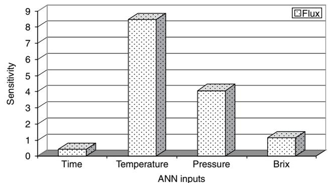
Fig. 4. Sensitivity of the best chosen ANN (4/6/1) toward the inputs for flux prediction.
