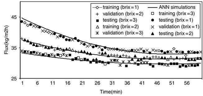
Fig. 2. Dynamic prediction of permeate flux during nanofiltration of sugar beet press water in different concentrations. Lines show the ANN prediction and symbols show the experimental data that was used for training (■), validating (×) and testing (○). ANN used: 4/6/1. Training points/validation points/testing points: 243/648/729 (operating conditions: TMP = 20 bar and T = 40°C).
