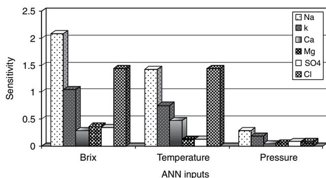
Fig. 5. Sensitivity of the best selected ANN (3/16/1) toward the inputs for prediction of ionic compounds rejection.
