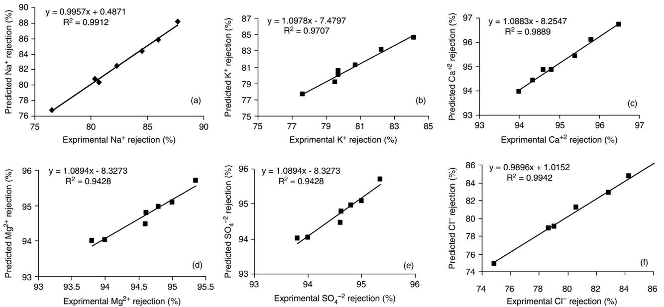
Fig. 3. Experimental and predicted ionic compounds rejections of sugar beet press water nanofiltration. ANN used: 3/16/1. Training points/validation points/testing points: 81/40/41.
