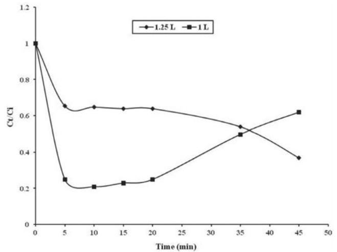
Fig. 4. Effect of volume of solution on rate of defluoridation of NaF solution (AR grade),  $C_i = 21.27$  mg l<sup>-1</sup>, seven bipolar electrodes, speed of agitation = 400 rpm, current = 250 mA, voltage = 10.5 V.
