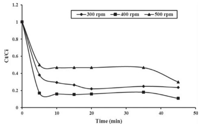
Fig. 3. Effect of speed of agitation on rate of defluoridation of NaF solution (AR grade),  $C_i = 42.17$  mg  $l^{-1}$ , volume of solution = 1 l, seven bipolar electrodes, current = 250 mA, voltage = 10.5 V.
