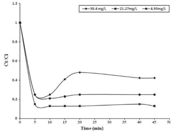
Fig. 2. Effect of initial concentration of fluoride in different commercial NaF solutions on rate of defluoridation,  $C_i = 30.4$ – $4.93$  mg  $l^{-1}$ , volume of solution = 1 l, seven bipolar electrodes, speed of agitation = 400 rpm, current = 250 mA, voltage = 10.5 V.
