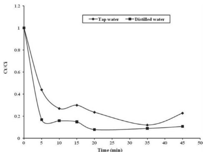
Fig. 5. Effect of presence or absence of coexisting ions on rate of defluoridation of NaF solution (AR grade),  $C_i = 42.17 \text{ mg l}^{-1}$ , volume of solution = 1 l, seven bipolar electrodes, speed of agitation = 400 rpm, current = 250 mA, voltage = 10.5 V.
