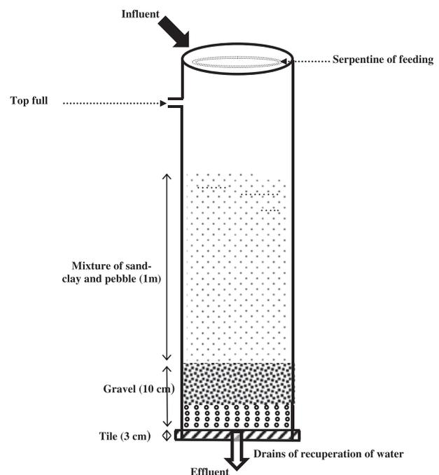
Fig. 1. Scheme of filtration column.
