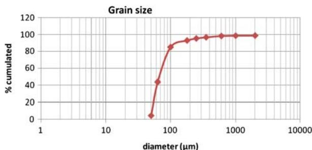
Fig. 2. Grain size of used sand.
