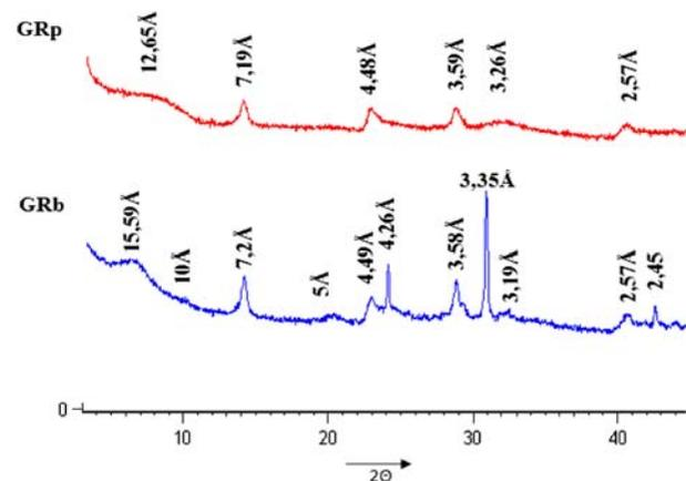
Fig. 4. XRD spectrum of natural clay, GRp: purified; GRb: raw.
