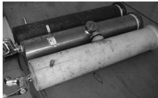
Fig. 1. Static pipe section reactor.
