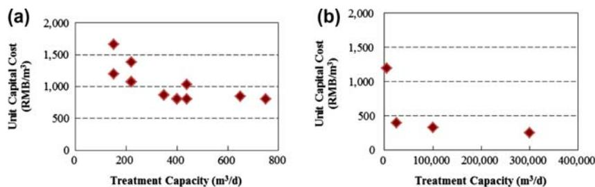
Fig. 10. Unit capital costs for a range of plant sizes (a) Omexell/Dow and (b) Litree.
