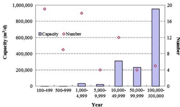
Fig. 3. Scale distribution of membrane plants in China (>100 m<sup>3</sup>/d).
