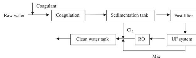
Fig. 9. Flow diagram of Kaotan Waterworks (300,000 m<sup>3</sup>/d).
