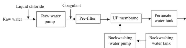
Fig. 8. Flow diagram of Ducun drinking water plant (10,000 m<sup>3</sup>/d).
