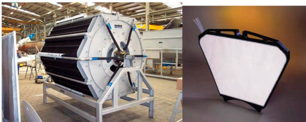
Fig. 2. The VRM membrane holder and a membrane module cassette.
