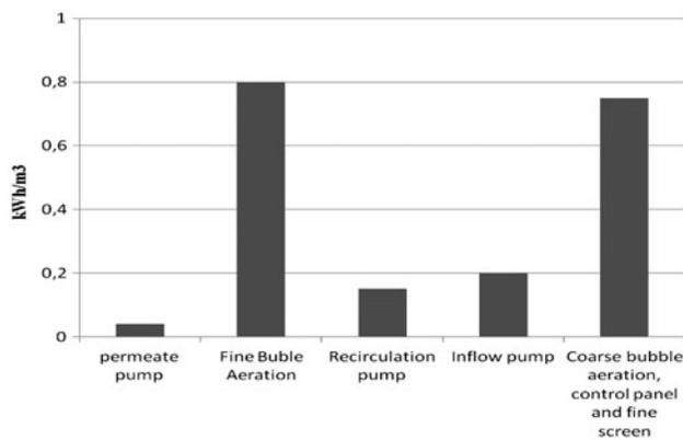
Fig. 8. Normalized energy consumption by each device making up the VRM plant.
