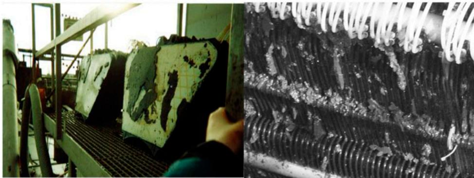
Fig. 9. Sludge layer on membrane plates and filled inter-plate spaces.
