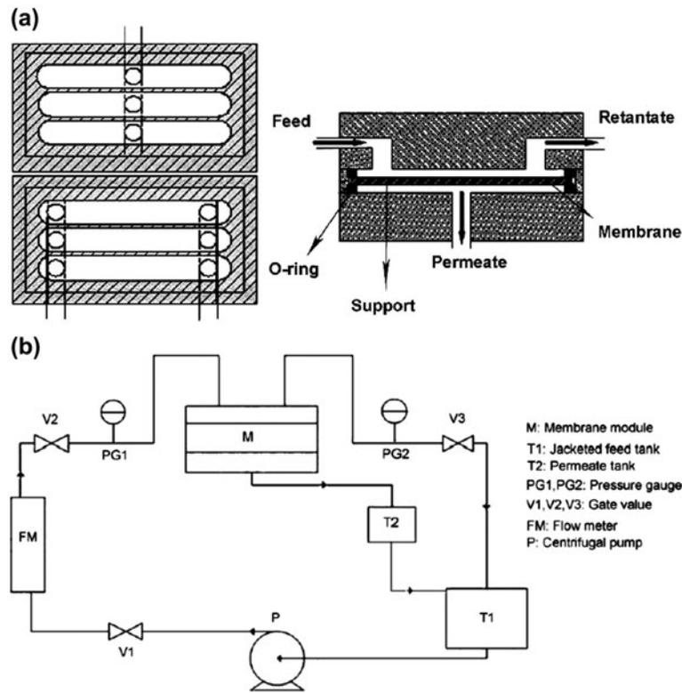
Fig. 2. (a) UF module and (b) diagram of UF experimental setup.
