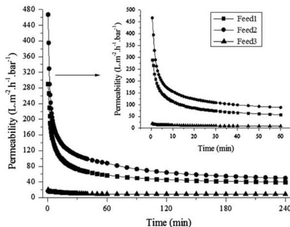
Fig. 4. Membrane permeability variations vs time for feed 1, feed 2, and feed 3 throughout 4 and 1 h of the process of UF.
