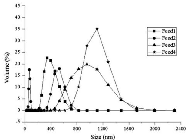
Fig. 1. Size distribution of particles for the all feeds.
