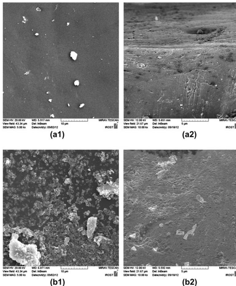
Fig. 5. SEM images of PAN350 membrane, formed cake layer and internal blockage, (a) fresh membrane before UF process, (b) resulted from UF process for feed 1, (c) resulted from UF process for feed 2, (d) resulted from UF process for feed 3, and (e) resulted from UF process for feed 4.
