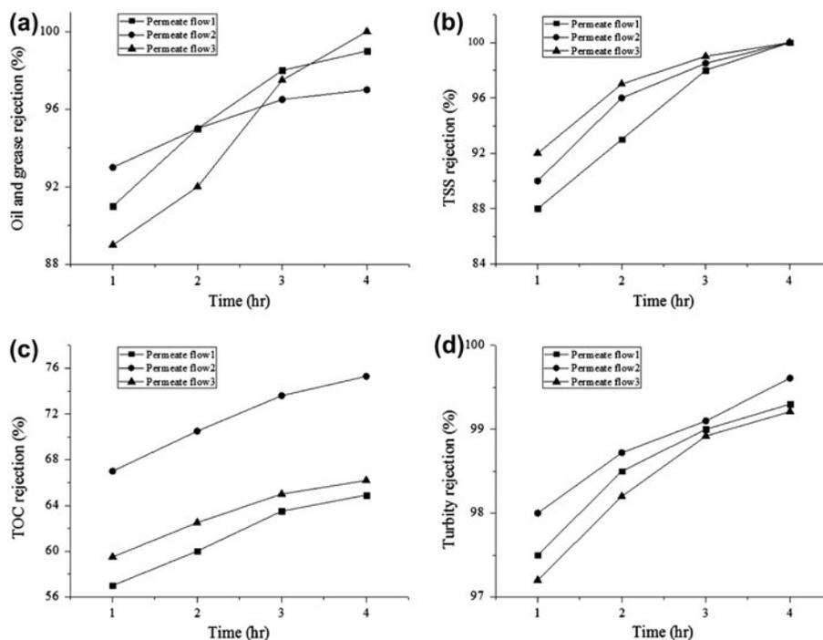
Fig. 3. Variation of (a) oil and grease, (b) TSS, (c) TOC, and (d) turbidity rejections vs time at optimum conditions during 4 h long experiments for three permeate flows 1, 2, and 3.
