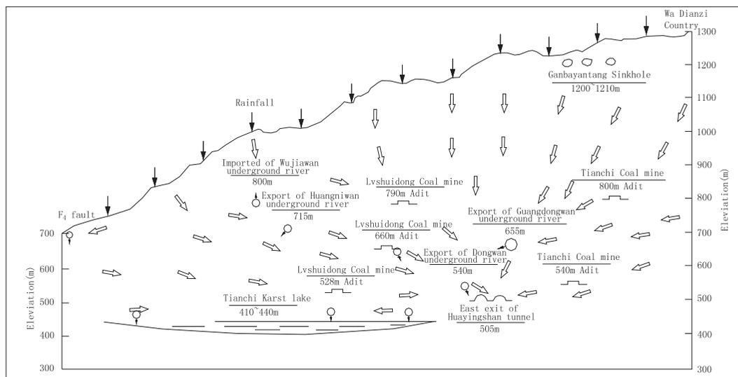
Fig. 10. Change in groundwater flow due to coal mining and tunnel construction in Huaying mountain.
