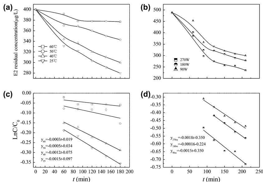
Fig. 1. Degradation of E2 by pure ultrasound process, and first-order kinetic models (frequency: 20 kHz; power: 180 W; volume: 200 mL; E2 initial concentration:  $400 \mu\text{g L}^{-1}$ ; pH: 7.05; (a), (c) temperature influence; and (b), (d) power influence).
