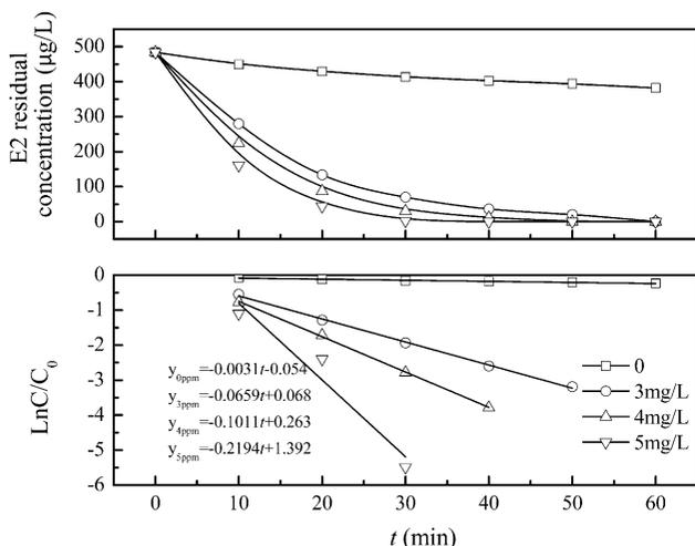
Fig. 2. Oxidative enhancing effect and first-order kinetics models of  $\text{KMnO}_4$  on the degradation of E2 in the ultrasound/ $\text{KMnO}_4$  process (frequency: 20 kHz; power: 270 W; volume: 200 mL; E2 initial concentration:  $484 \mu\text{g L}^{-1}$ ; pH: 7.38; and temperature:  $25 \pm 1^\circ\text{C}$ ).
