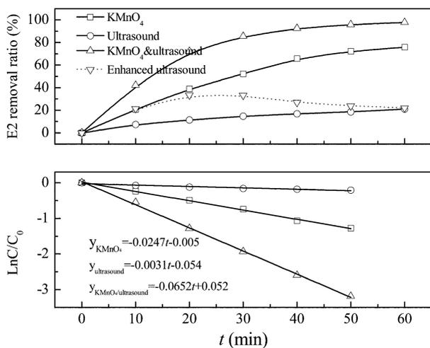
Fig. 3. First-order kinetics models and degradation efficiency of E2 by three processes: pure  $\text{KMnO}_4$ , pure ultrasound, and ultrasound/ $\text{KMnO}_4$  (frequency: 20 kHz; power: 270 W; volume: 200 mL; E2 initial concentration:  $484 \mu\text{g L}^{-1}$ ; pH: 6.86; and temperature:  $25 \pm 1^\circ\text{C}$ ).
