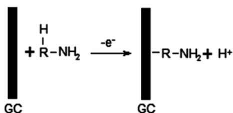
Scheme 1. Proposed mechanism for layer formation through the ring.
