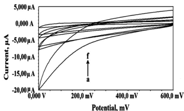
Fig. 4. Cyclic voltammograms of 1.0 mM of  $\text{Fe}(\text{CN})_6^{3-}$  in BR buffer solutions of various pH values at the 1AIn/GC electrode. Corresponding pH values are: (a) 2.0, (b) 4.0, (c) 6.0, (d) 7.0, (e) 9.0 and (f) 11.0. The scan rate was 100 mV/s vs. Ag/AgCl/  $\text{KCl}_{\text{sat}}$ .
