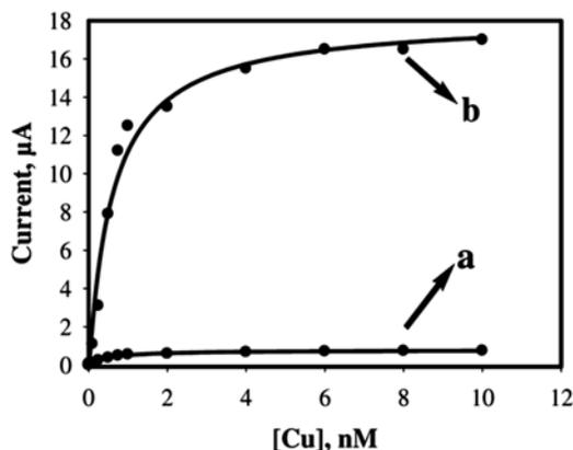
Fig. 6. Amperometric responses of the (a) bare and (b) 1AIn/GC electrodes at  $-400$  mV vs.  $\text{Ag}/\text{AgCl}/\text{KCl}_{\text{sat}}$  upon successive addition of  $0.001$ – $10$  nM of Cu(II).
