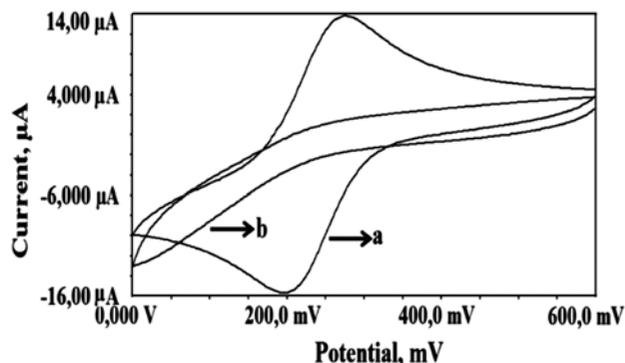
Fig. 2. The cyclic voltammograms of 1.0 mM of  $\text{Fe}(\text{CN})_6^{3-}$  in BR buffer solution, pH 2.0, at the (a) bare GC and (b) 1AIn/GC electrodes. The scan rate was 100 mV/s vs.  $\text{Ag}/\text{AgCl}/\text{KCl}_{\text{sat}}$ .
