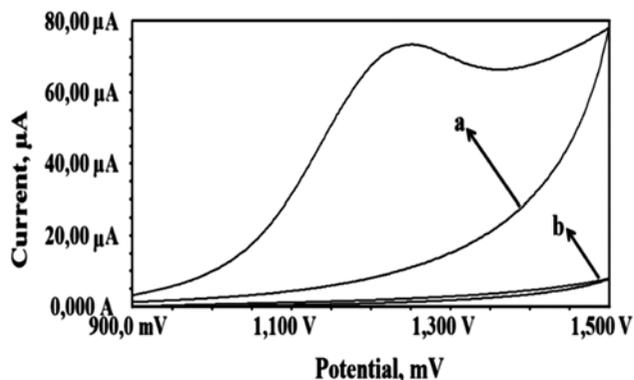
Fig. 1. Cyclic voltammograms of 10.0 mM of 1AIn and 100 mM of TBATFB in  $\text{CH}_3\text{CN}$  at the bare GC electrode: (a) 1st and (b) 30th cycles. The scan rate was 100 mV/s vs.  $\text{Ag}/\text{Ag}^+/\text{AgNO}_3$ .
