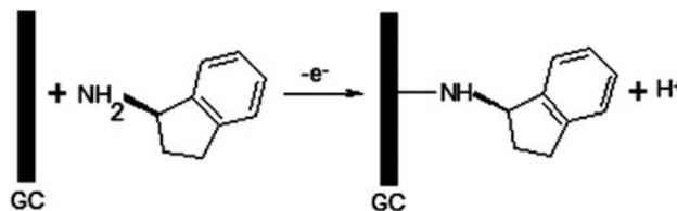
Scheme 2. Proposed mechanism for layer formation through amine oxidation.
