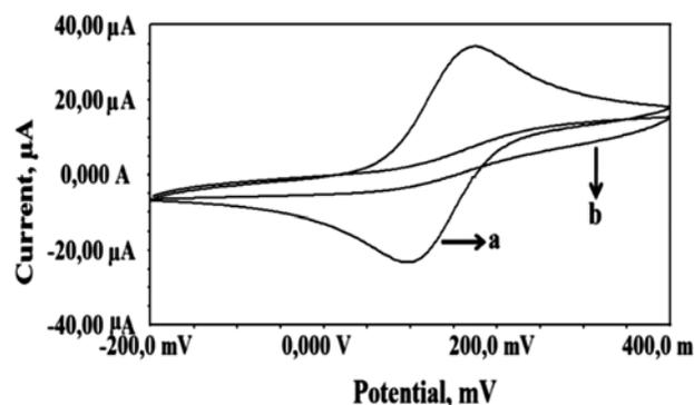
Fig. 3. The cyclic voltammograms of 1.0 mM of ferrocene in  $\text{CH}_3\text{CN}$  containing 100 mM of TBATFB at the (a) bare GC and (b) 1AIn/GC electrodes. The scan rate was 100 mV/s vs.  $\text{Ag}/\text{Ag}^+/\text{AgNO}_3$ .
